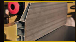
SIDE PLATE Oversized side plate can be used in the horizontal or vertical position.
