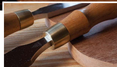
Hidden strength. The closed ferrule of the Blue Spruce chisel hides a stepped tang that protects the handle from splitting.
