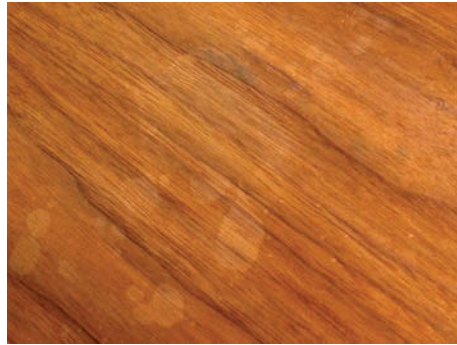
Watco watermarks. Watco Danish Oil claims better protection because the finish polymerizes "in" the wood. Here, I left puddles of water on three coats of dried Watco for just more than a minute. It's clear that resistance to water penetration is very minimal.
