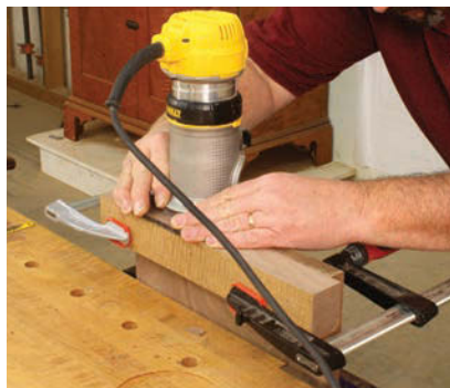
Quick work. A sacrificial support and a router with a straight bit easily hogs away waste from between your dovetail pins.
