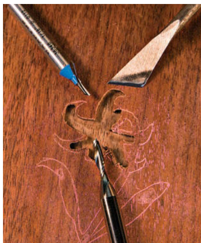
Choose your tools. To cut the cavity for the inlay, use a succession of tools. At bottom is a \frac{1}{8} " bit used to clear the field. At top left is a \frac{1}{16} " bit that can get into tighter spots. Finish off with small chisels and knives (top, right). Cut right up to the scribe lines and keep the recess a consistent depth.
