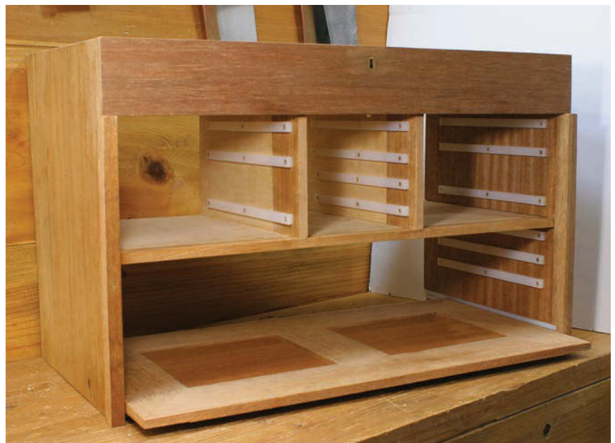
No nails, two tails. My machinist's-style tool chest is screwed together (with the exception of two sliding dovetails for the horizontal divider). The filler strips have yet to be planed to match the case. Though a modern woodworker may cut parts to final size from the start, the traditional approach is to fit parts piece by piece.
