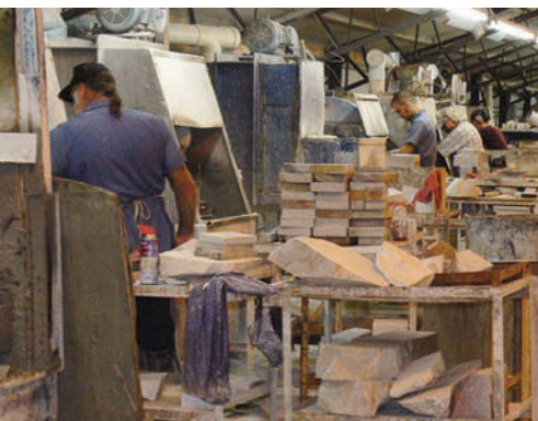
Cut to size. To further reduce the stones’ size, they’re cut on a row of 36”- and 18”-diameter saws. The enclosures help to contain the dust.
