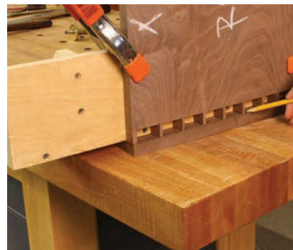
Simple jig for layout transfer. A 90° jig holds the pin board as you transfer your layout to the tail board.
