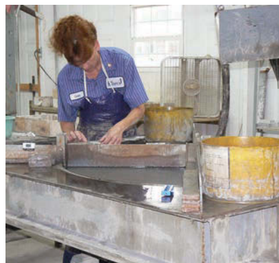
Rotating tables. Silicon carbide in progressively finer grits is used to grind the stones smooth on rotating lapidary tables.
