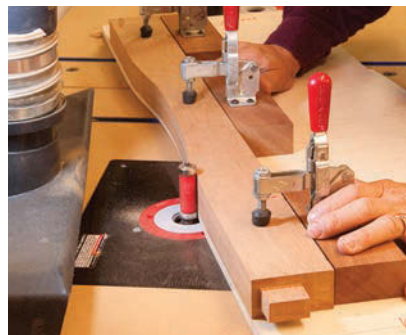
Ramp up. Extra length at the beginning and end of the curved pattern guarantees a good cut with the router.
