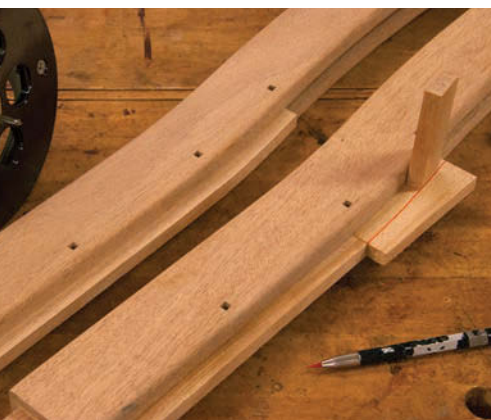
Two step. The exposed tongue is in two pieces, use a spacer to gauge the sizing of the curved portion.
