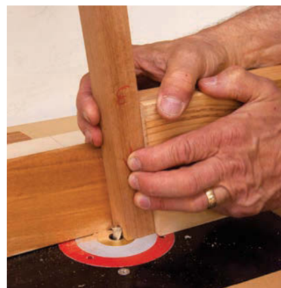
In the saddle. The slots in the ends of the spindles fit over the tongues in the rails. Angled stock safely guides the workpiece.
