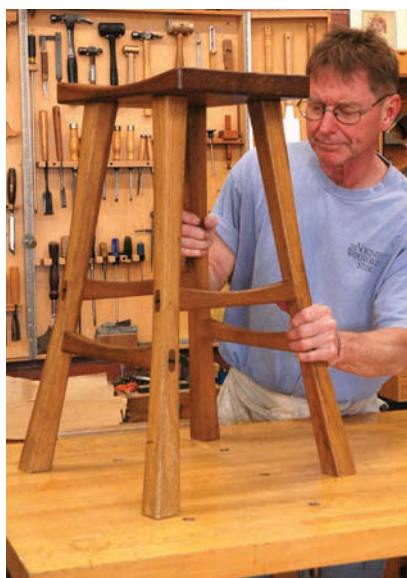
Bench flat is flat. When the stool no longer rocks on your bench, your work is done. Your four legs have been tried and trued.
