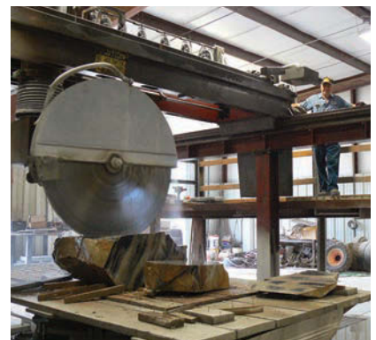
Now that's a saw. Large chunks of stone are cut down to a workable size on this 54"-diameter stone saw.
