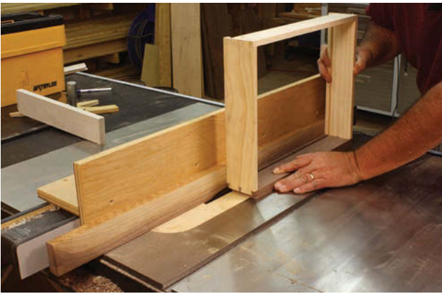
Hold tear-out at bay. Rabbits cut using a dado stack are less apt to tear-out, but you should still plane the two ends before the sides.
