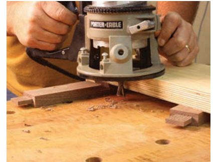
Setup for sliding dovetails. Sliding dovetail sockets on the base stretchers are easy when you install a 3/4" outside-diameter dovetail bit with a 3/4" outside-diameter guide bushing. Wherever the bushing travels, the bit will cut.
