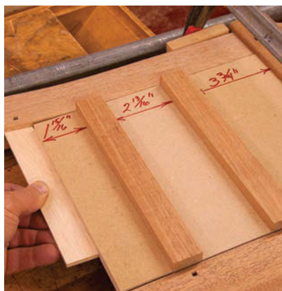
Spindle spacing. Cut spacers to locate the vertical spindles and mark the ends for length and for the correct angle.
