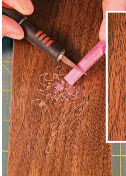
Chalk it up. Remove the inlay and sprinkle chalk dust across the scribed guidelines. Using chalk of a contrasting color makes it easy to spot your lines.
