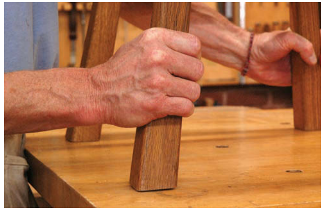
Find the culprits. Check for twist using the bench as a flat reference surface. Pushing on opposing corners will identify which legs are longer, mark those with chalk.
