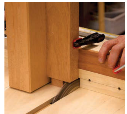
Smart setup. The vertical block attached to the sled allows the tenons to be machined vertically without adjusting the blade height.
