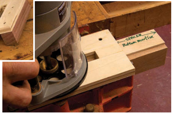
Under control. The spacer locates the template the identical distance from the end of each leg.
