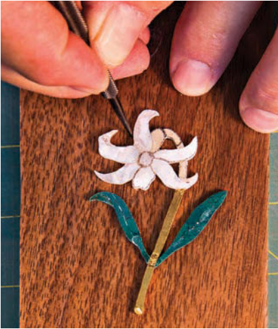
Mark it out. Align the inlay on the workpiece and glue it down using Duco Cement. Then scribe around the outside of the pattern.
