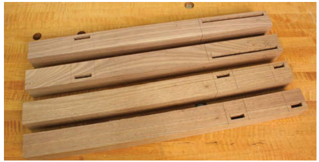
Flush fit. The 1/4"-wide x 1"-deep mortises are positioned so the rails fit flush to the outside face of your legs.
