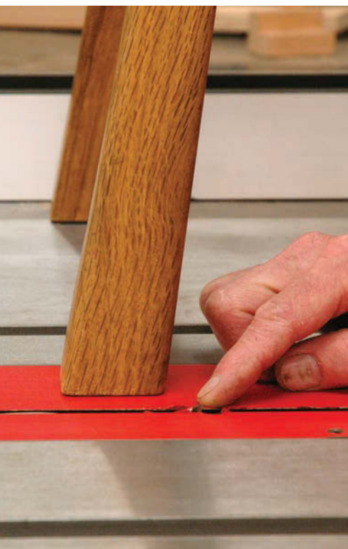
Barely there. Set the blade height for a mere \frac{1}{64} " to \frac{1}{32} ". You should just feel the blade coming up out of the table throat plate insert. A saw blade with a flat-top grind works best.
