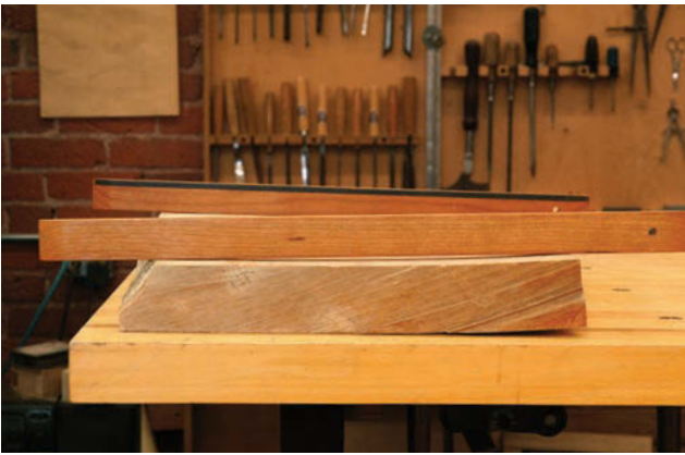
Twisted board, twisted legs. This twisted board illustrates just how a four-legged piece can also twist. There are two opposing high sides vs. two low ones. The winding sticks show what's high and low.
