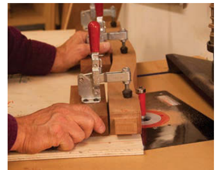
Ramp down. The extra width of the pattern provides room for placing clamps and keeps your hands a safe distance from the bit.
