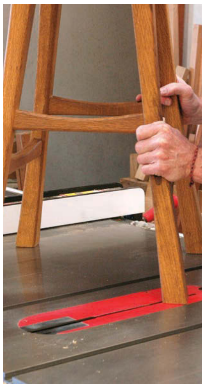
Quick shave. True a leg on the table saw the quick and easy way. Make sure the blade is set for a very small cut. Laterally move one of the longer legs slowly over the spinning blade.
