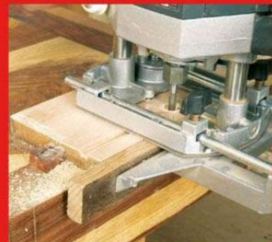
Reduce the risk of tear-out by adding a timber offcut to the side fence.
