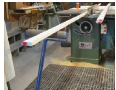
When ripping long boards, support them with extension rollers to keep the work piece level and in line to the saw blade.
