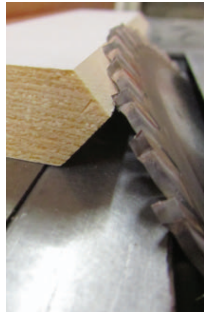
Cutting the opposite edges at 45 degrees provides the decorative beveled edge.
