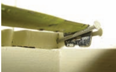
When working alone and measuring long distances, insert a nail close to the opposite wall and hook your tape onto it.
