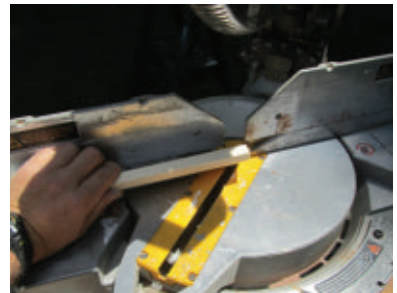
The molding was cut on a miter saw using the "upside-down and backward" method.
