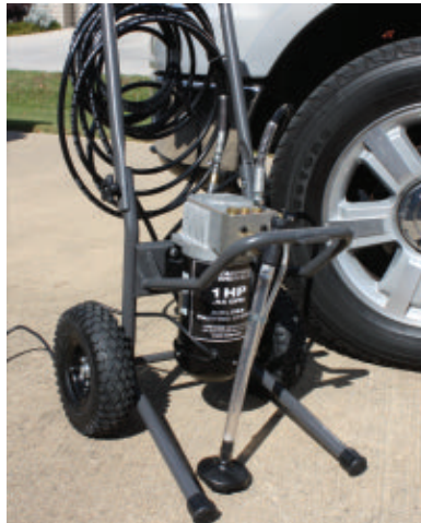
This project utilized Defy Extreme Wood Stain, which was sprayed on with a heavy-duty 1-HP Campbell Hausfeld airless sprayer.
