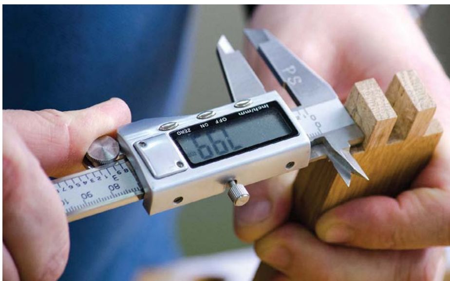
A GemRed digital Vernier calliper checking thickness
