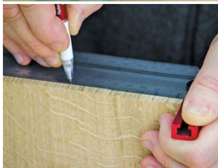
Using an INCRA T-rule for progressive markings
