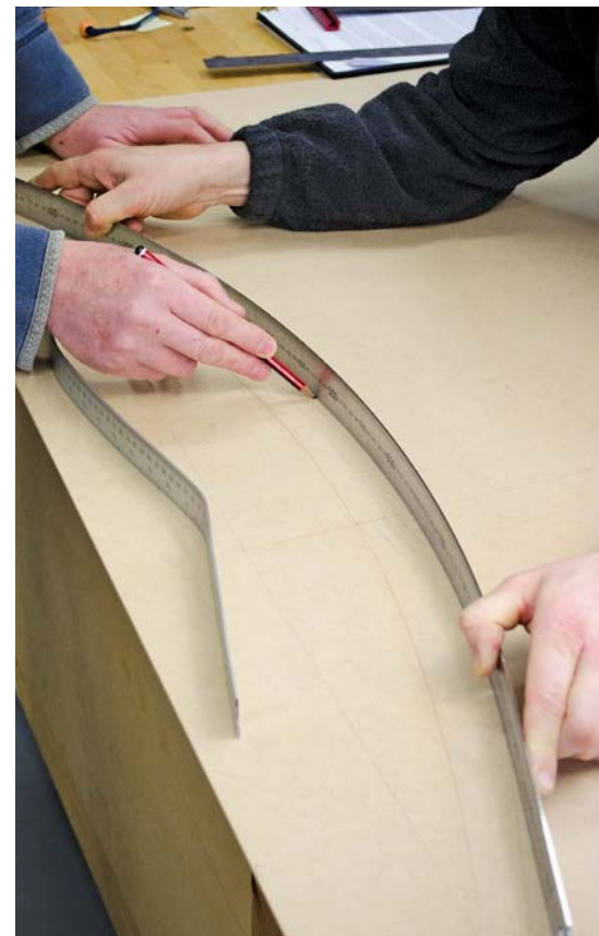
Bending a rule and a bent rule
