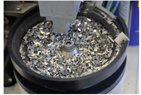
Carbide tips sit in a rotating sorting tray
