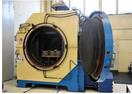
Blades entering the hydrogen chamber when they will be annealed
