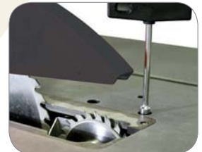
Height & side setting of the scoring blade conveniently accomplished with the tool provided.
