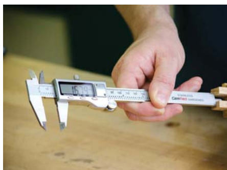
A GemRed digital Vernier calliper checking depth
