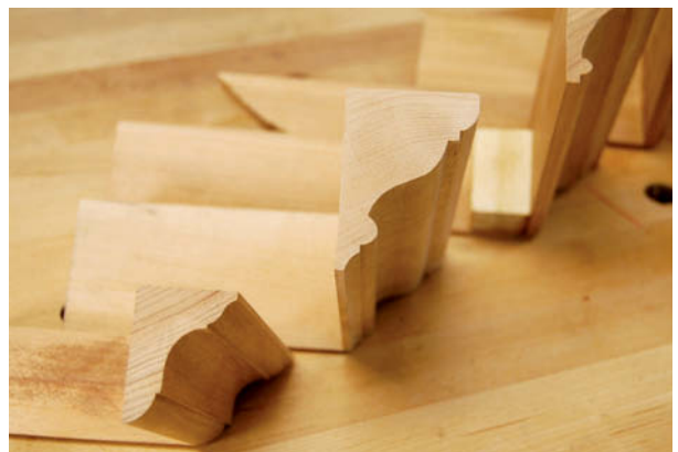
Molding planes allow duplication of virtually any profile.
