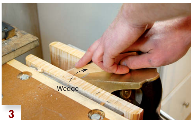
3 The plane's wedge is tapered to fit the housing so it will lock the blade's shaft in position.
