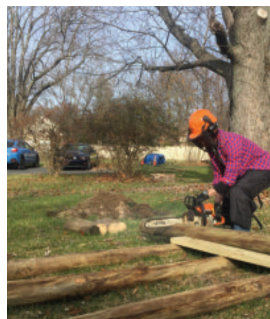
The sawbuck stabilizes the work and keeps the saw out of the dirt for clean, fast cuts.
