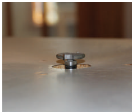
Use a tongue-and-groove router bit to shape the ends of the boards.
