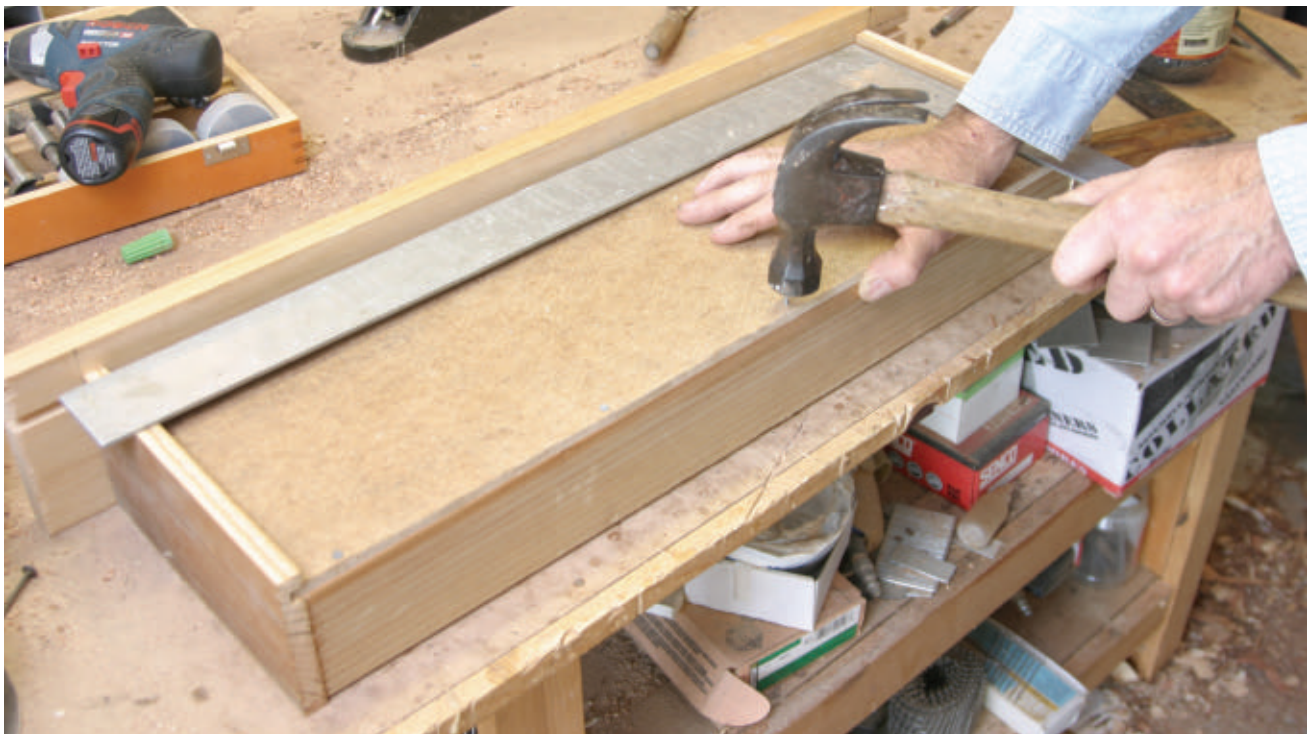
Assemble the drawer. The bottom is held in dadoes in the front and sides, and fastened down to the bottom edge of the back with flat-head nails. Make sure the drawer is assembled square.
