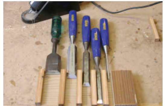
Wood chisels are held in a holder of 1/2" stock. Glue the spacers between the chisels to the front of the holder with hot-melt glue.
