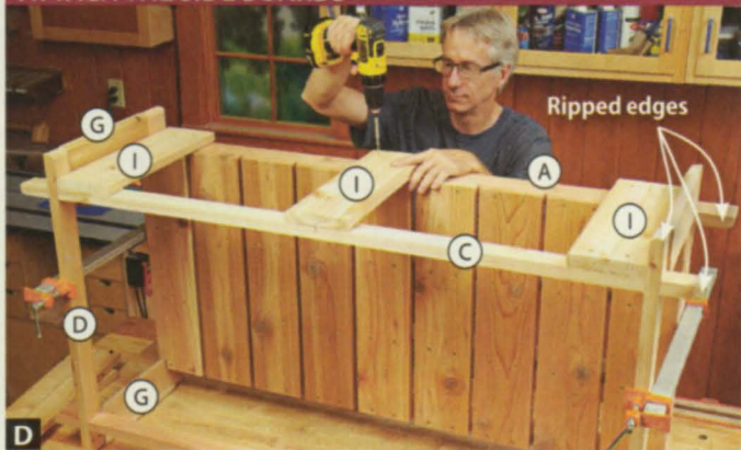
D Screw a side board (I) flush to the rails (A, C) at each end and one centered between the ends. Space the remaining side boards evenly in the gaps.
