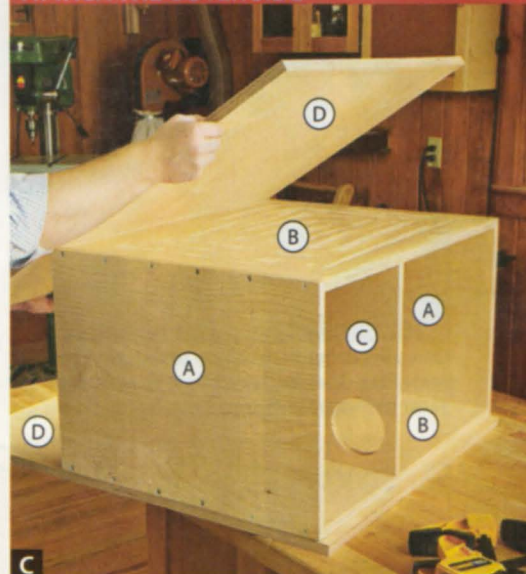
C Apply glue to the outer faces of the inner sides (B). Position the outer sides (D) and clamp or weight the pieces until the glue has dried.
