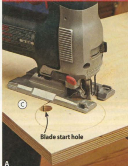
A Mark the 4" hole in the baffle (C) with a compass, bore a \frac{3}{4} " blade start hole near its inside edge, and cut along the marked line with a jigsaw.
