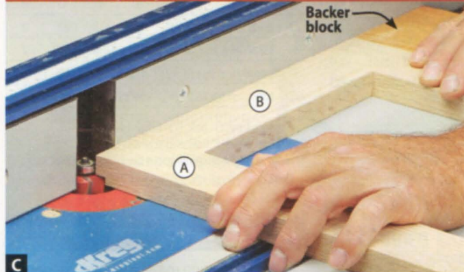
Employ the same tenon-cutting technique used on the ends of the support rails (B) to form a tongue along one short edge of both support frames (A/B).
