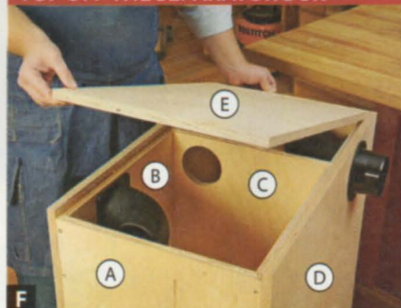
F Apply a bead of glue to mating surfaces, align the separator-box top (E), and attach with countersunk 1½" screws.
