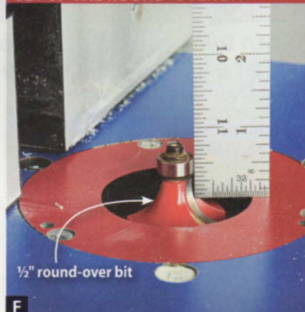
F Adjust the top of the bit's cutting edge \frac{5}{16} " above the router table prior to rounding over the top caps (L) and panel-bottom trim (M).
