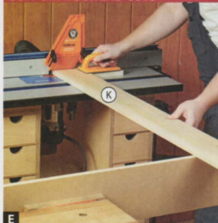
E Clamp a support board in a nearby bench vise or to a sawhorse to hold the bottom cap (K) level with the router table when routing the ends.
