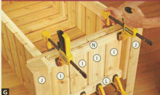
G To allow the side boards (I) to expand and contract, apply glue to only the center 2" of each side board; then clamp the trim (K, L, M, N) in place.
