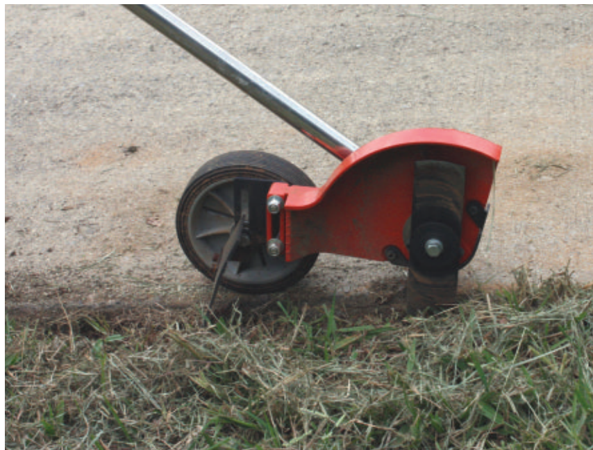
For single-wheeled edgers, keep the top of the blade tilted away from the hardscape when cutting.
