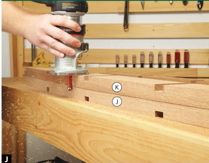
J Set the depth of the pattern/flush-trim bit so that the bit avoids the dadoes as it rides against the top back rail (J) to smooth the middle back rails (K).
