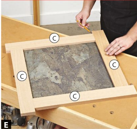
E Because tile dimensions can vary, arrange the top trim pieces (C) in an overlapping pattern around the 18" tile to mark each board's actual length.
