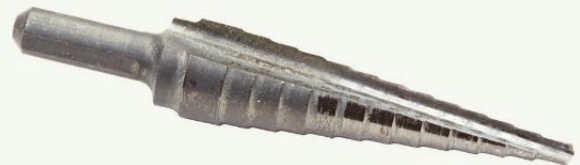
To easily choose the correct diameter, this stepped drill bit (Milwaukee Tools, no. 48-89-9100, milwaukeetool.com) has etched measurements at each of its progressively larger diameters.
