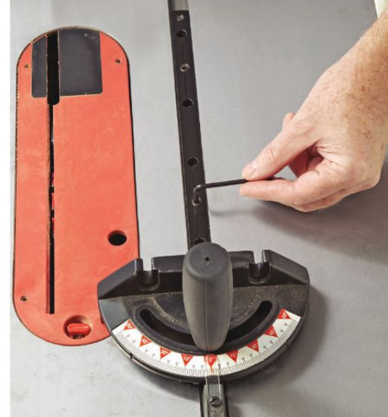
Jet's miter gauge can be adjusted to fit more tightly or loosely in the slot by changing the slotted bar's width via three setscrews.
