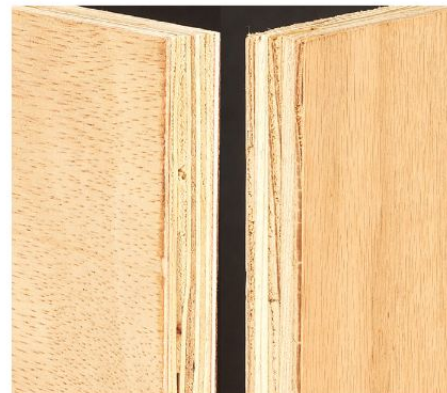
Though it costs 50 percent more, the plywood on the right eliminates uneven core veneers, voids, and a distinct curl that could impact your success.
