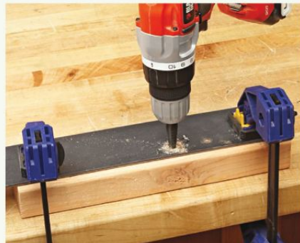
With the steel plate and a backer board clamped to your worksurface, drill \frac{3}{8} ", \frac{1}{32} ", and \frac{5}{16} " holes through the steel plate.
