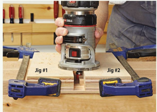
Make multiple shallow passes to complete the dado, running the bearing first along one fence and then back along the other.
