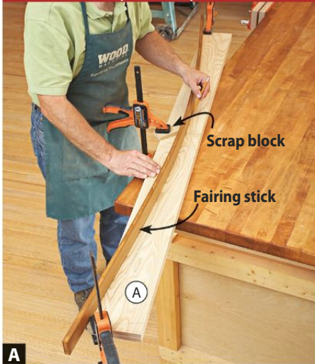
A To draw an even curve on the tower side (A) and arm side (D) blanks, bend an MDF fairing stick and hold it in place with clamps and a piece of scrap.
