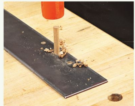
With the dowel-plate hole aligned over a dog hole, pound the blank first through the \frac{3}{8} " hole, then the \frac{1}{32} " and \frac{5}{16} " holes.
