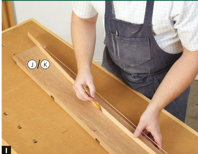
I A thin scrap of wood (fairing stick) tensioned to intersect the curve's top and ends, makes a perfect arch for laying out the curves of the back rails (J, K).
