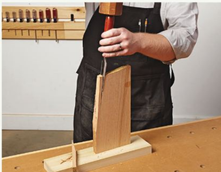
Chop lengths of your project stock from a piece of scrap, splitting the wood along the grain. Plane, file, or sand the dowel blanks to roughly \frac{3}{8} " diameter.
