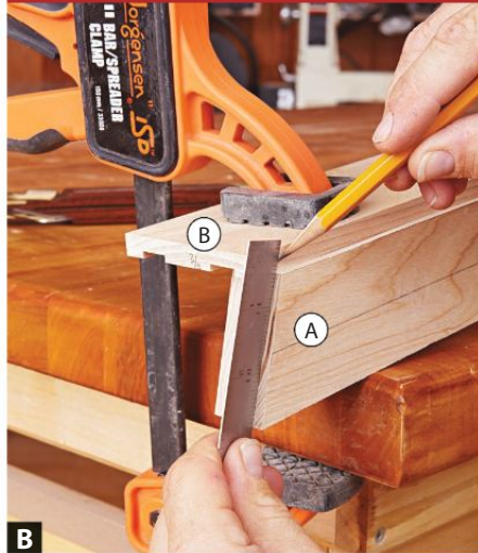
B Use a straightedge against the angled ends of the tower sides (A) to mark the angle of the tower back (B) end.
