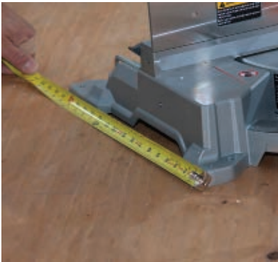
Measure the base of the miter saw to determine the width of the saw table.
