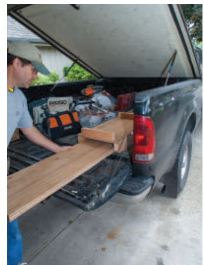
We build most of our saw tables so they can fit in a truck bed. The wing boards and our levels go under the table. We stack tools on top of the table.
