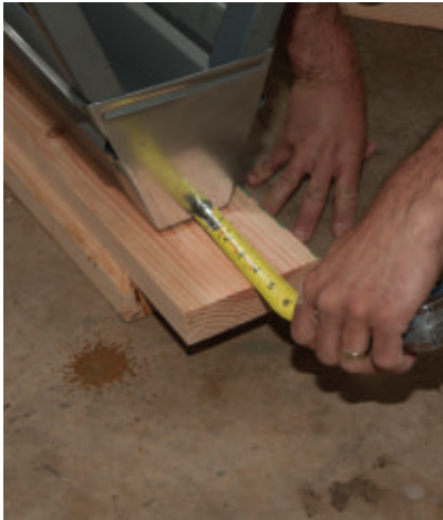
The 2x6s we add to the tops of folding saw horses are a few inches longer than the horses for added material stacking.
