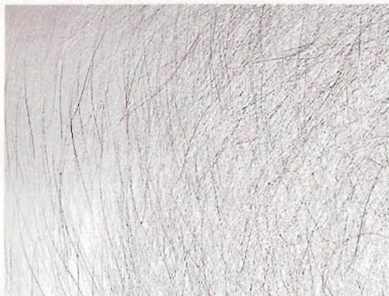
▲ Rotary motion mode moves the disc in a large, circular orbit. This mode is perfect for aggressive stock removal and rough work.
