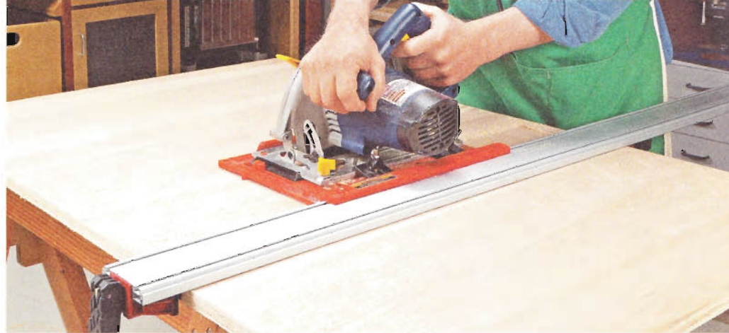
▲ The Wide Track Saw Guide from Bora attaches to the base of your circular saw. The guide rides along a T-track in the straightedge to produce straight, accurate cuts.
