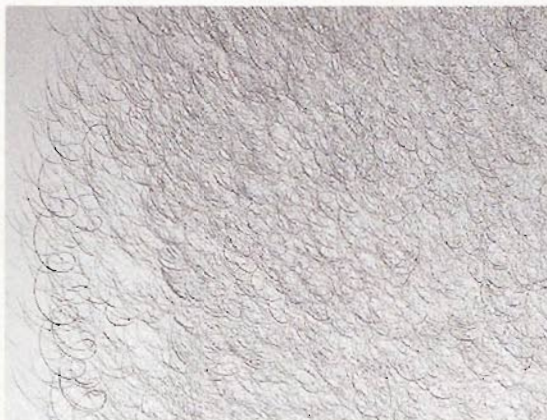
▲ When switched to eccentric motion mode, the pad moves in very small, tight circles. This scratch pattern is better for finish work.
