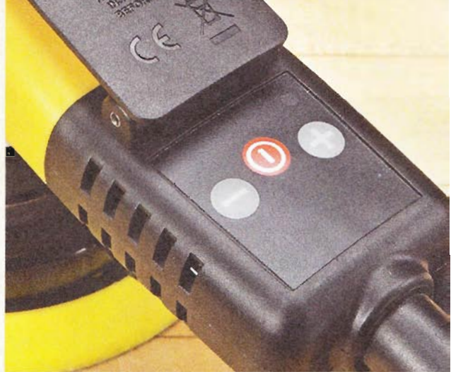
▲ The speed controls on the CEROS are located just behind the paddle switch.
