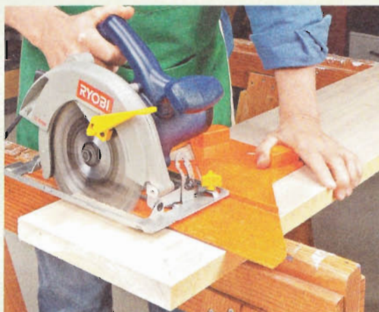
▲ Once the Pro-Cut is trimmed to size, all you do is line it up with the cut line on the board and hold it firmly as you begin cutting.
