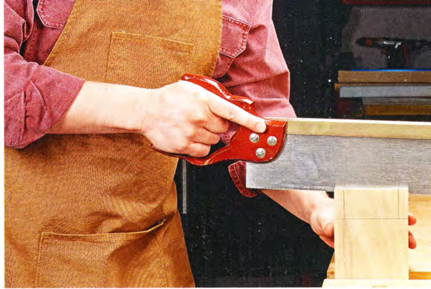
▲ Good posture not only helps your back, but your woodworking, too. Stand as straight as possible with your elbows close to your body.
