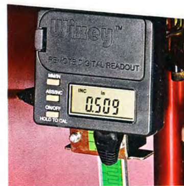
▲ A sensor that's attached to the router lift's carriage gives you a precise height reading on the display panel.
