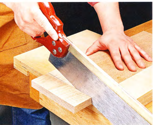
▲ A bench hook consists of a base and a pair of cleats. One cleat fits on the underside and anchors to the edge of your bench. The other is a fence for the workpiece.
