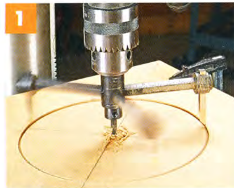
▲ These drill press circle cutters work well for making a hole template in \frac{1}{4} " hardboard. Use a low RPM setting.
