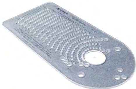
▲ Commercial trammels (like this one from Jasper) are available that fit different routers and cut virtually any radius.
