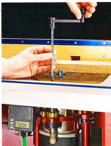
▲ A sensor that's attached to the router lift's carriage gives you a precise height reading on the display panel.
