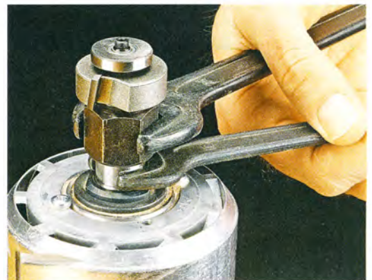
▲ It's possible to over-tighten a router bit in the collet. By using one hand to tighten, you can avoid over-tightening, as well as pinched fingers.
