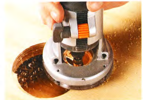
▲ After rabbeting the opening, run the pattern bit's bearing against the rabbeted portion of the hole to enlarge it.
