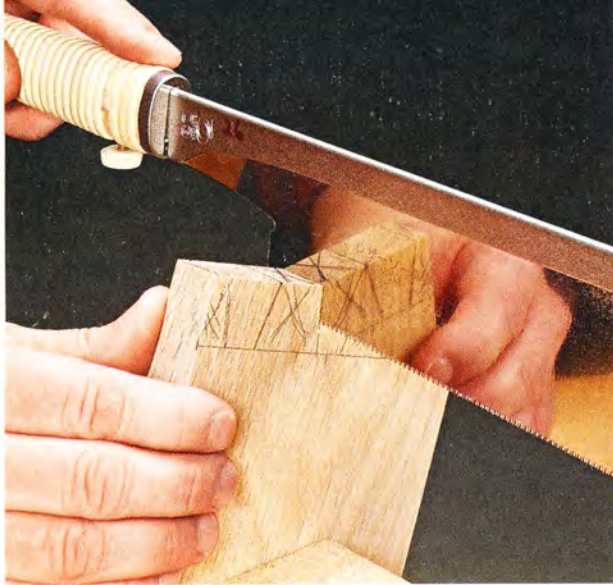
▲ For angled cuts like dovetails, tilt the workpiece in the vise to match the angle. Then you can make a straight cut.
