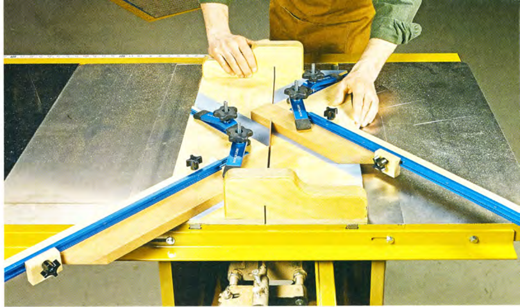
▲ Be sure to keep the frame pieces oriented in the right direction when making the second and third passes. Labeling the pieces after the first cut helps to keep them in order.
