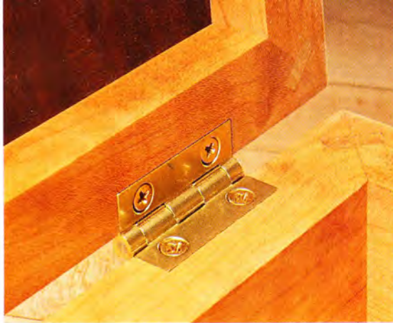
▲ While they can be surface-mounted, these Brusso stop hinges are easy to install in a mortise. The square knuckle has a built-in stop.
