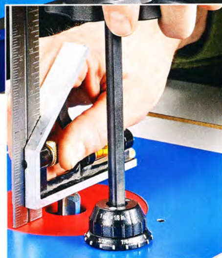
▲ Some router models come with built-in "above-the-table height adjustment." An included knob makes this easy.
