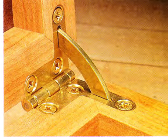
▲ Quadrant hinges require precise alignment to install. The arc-shaped support arm holds the lid open at 95°.
