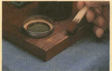
Touch-up. When sanding between coats, it's possible to cut through the stain. Use a small sponge "dabber" as a touch-up tool.
