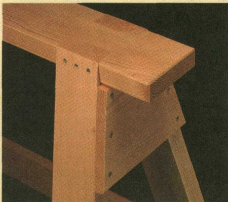
A The notches cut in the top piece angle the legs outward in two directions. Gussets and stretchers brace the legs to make the sawhorse strong and sturdy.
