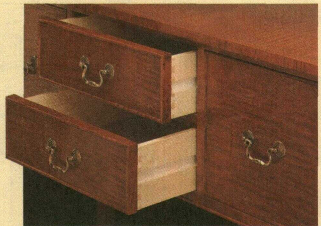
A This sideboard is a mix of old and new. The top and drawer fronts are covered with traditional veneer, but the core is modern plywood. Also, the drawers are joined with dovetails — that are cut with a router and a jig.
