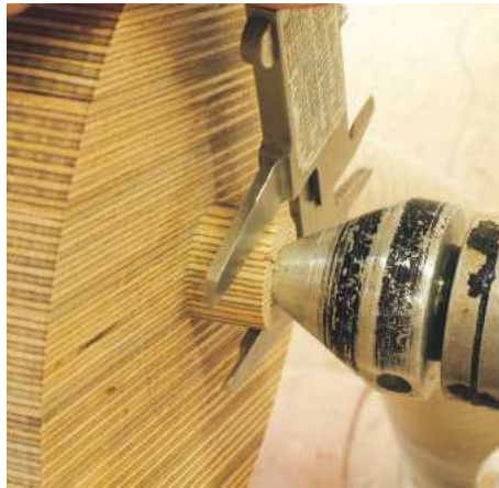
▲ Pic.20 The waste area at the top of the lamp is turned down to the diameter of the brass plate that will hold the lamp fitting. Watch out for the plywood splitting at the top
