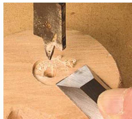
▲ Pic. 3 You have to be super-careful when trimming the counterbore
