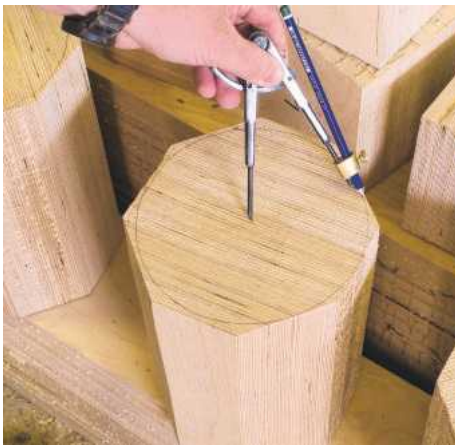
▲ Pic.4 He likes to get as close to his finish size as possible, because it's easier to cut away the wood with the saw than to turn it. He picks the middle strip of the ply and draws a circle to find the centre
