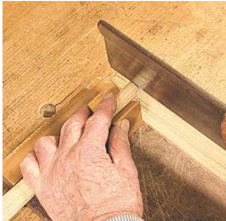
▲ Pic. 5 Saw a very shallow kerf to form the shoulder line
