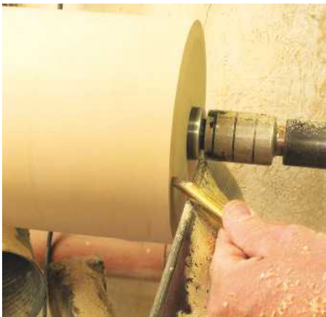
▲ Pic.13 The base needs to be slightly undercut to sit properly. Use a gouge with a push cut, but do not undercut too much because the baize will then look odd on the bottom
