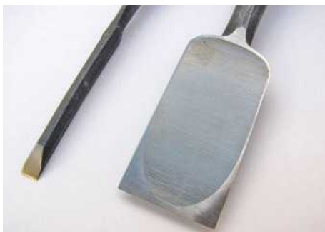
The hollow backs are typical of Japanese edge tools
