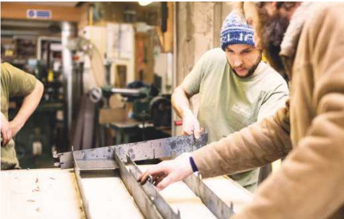
Assembling the custom-sloped frame which will convert the Wadkin thicknesser into a wedge-nesser
