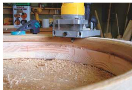
▲ Pic.14 Check the fit of the beading in the frame, then add a profile with a rounding over bit
