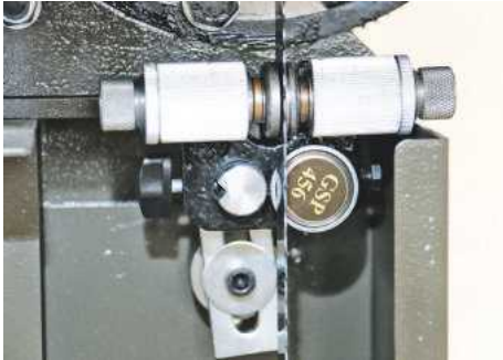
▲ The lower guides are easily accessible and are identical to the upper ones
