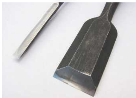
The single bevel is incredibly sharp
