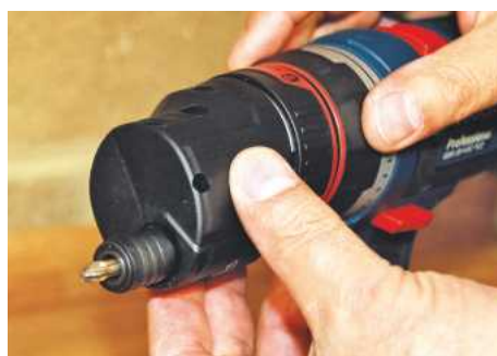
▲ You can rotate it to any position around the drill for different applications
