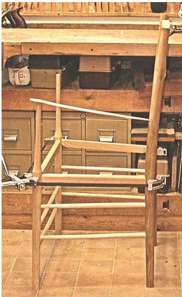
◀ Pic. 1 A steel band clamp temporarily holds the post & rail chair together while Jeff experiments with the arm's slope
