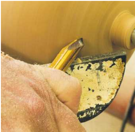
▲ Pic.19 Les doesn't like sharpening a tool that still has one of its cutting edges sharp, so will use a pull cut around the top so as to utilise both edges
