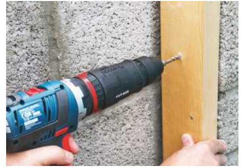
▲ The SDS chuck is powerful, quick and efficient for masonry work
