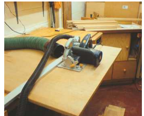
▲ Pic.2 The light circular saw, along with a clamp guide, is ideal for ripping the MDF to size
