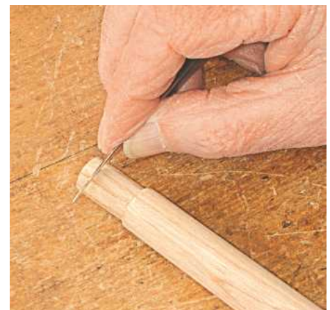
▲ Pic. 9 When tuning the tenon's fit, Jeff avoided scraping its tip
