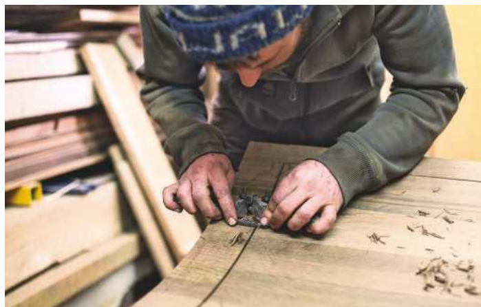
Cleaning up the front faces of the bar cupboard doors with a careful spokeshave
