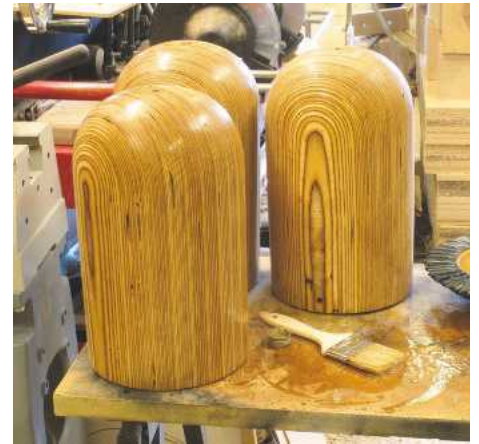
▲ Pic.30 Les experimented to find the best finish. Lacquer wasn't good on the end grain so he opted for hard wax oil, applying two coats with a light cut back between them
