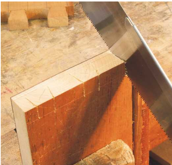
▲ Pic.8 Cutting the lapped pins
