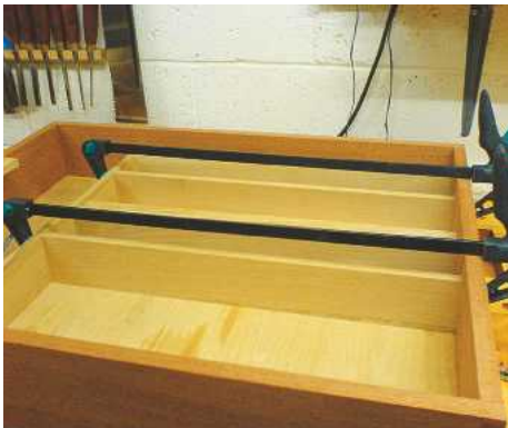
▲ Pic.11 A dry run is essential for this project, but you'll need quite a few clamps!
