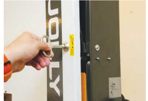
▲ Each door is microswitched but still has a lock to secure it
