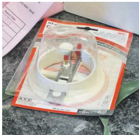
▲ Pic.35 The lamp bases do need to have baize on the bottom. The circle cutter will give you a perfect circle; scissors will not cut the baize clean enough
