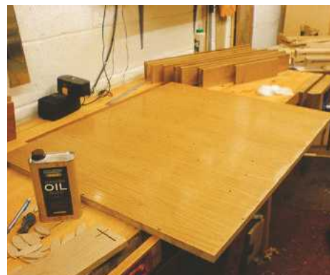
▲ Pic.16 Remove the MDF rear panel so you can drill and pre-finish it
