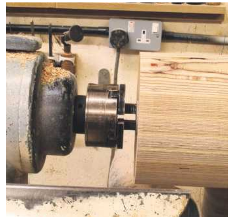
▲ Pic.15 Les has turned the base round. He likes to support the work on pin jaws, and these will hold the piece as he thins down the top. With increased tailstock pressure you could just drive off a cone
