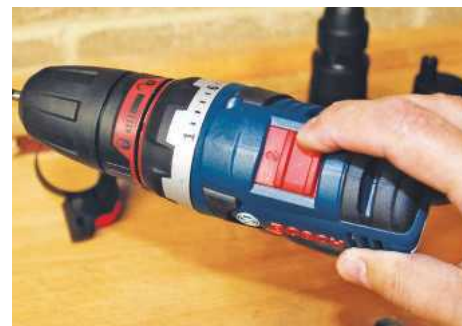
▲ The body has a standard 2-speed selector switch and torque collar
