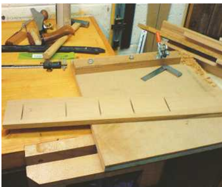
▲ Pic.14 ...so that the slots are exactly perpendicular to the sides
