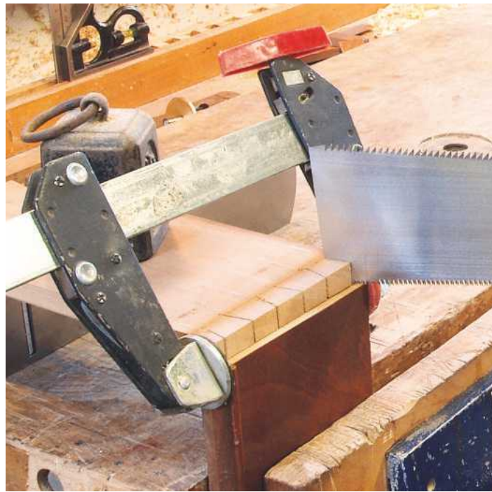
▲ Pic.7 Marking the saw cuts onto the pinboard in the old-fashioned way
