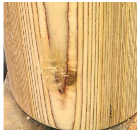
▲ Pic.27 Larger holes will need to be filled in two goes. This one is a remnant of a knot in the birch. Apply the filler by hand with the abrasive on a cork block
