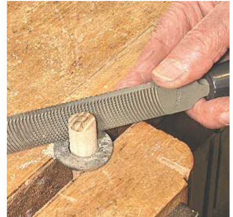
▲ Pic. 6 The washer protects the shoulder face while the file does its job
