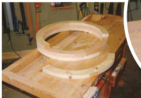
▲ Pic.6 Cut and mitre oversize segments for the final layer, using the frame as a base
