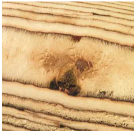
▲ Pic.14 Even though this is top-grade ply there is the likelihood of coming across defects in the wood. These don't seem to detract from the finished lamp base though
