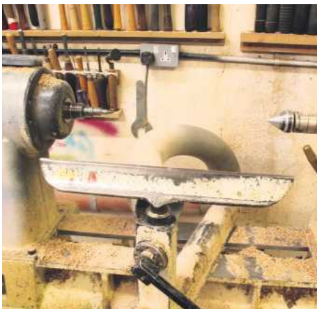
▲ Pic.7 Mounting the work between centres using the holes means a normal drive can't always be employed. Here Les is using Axminster's steeped drive but a counterbore drive would work as well
