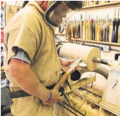
▲ Pic.10 The roughing gouge is braced to the side of the body and worked along the toolrest. Keeping the handle down low means the bevel is in contact with the wood
