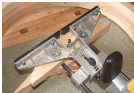
▲ Pic.9 Screw a piece of wood to the router fence and drill an 8mm hole, the trammel centre
