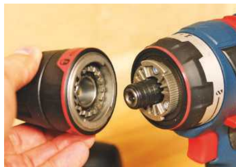
▲ Each chuck has a high-quality alloy connector that matches the connector on the drill
