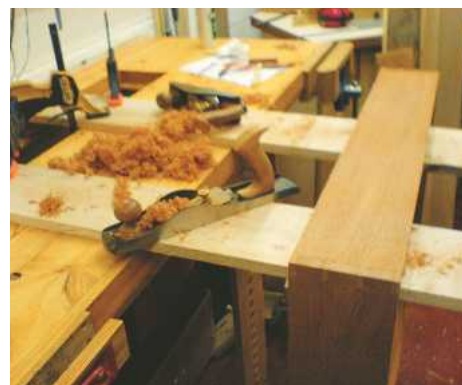
▲ Pic.10 Clean out the corners of the stopped rebates and the pin joints
