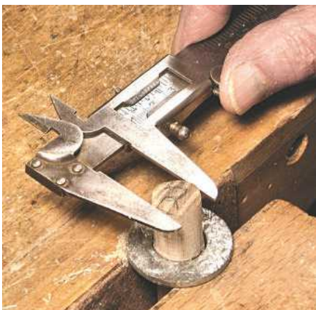
▲ Pic. 7 You need to check the filing with a Vernier calliper gauge
