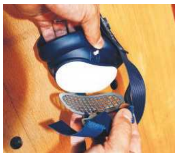
▲ Once released, the grille hinges back out of the way to gain access to the filter
