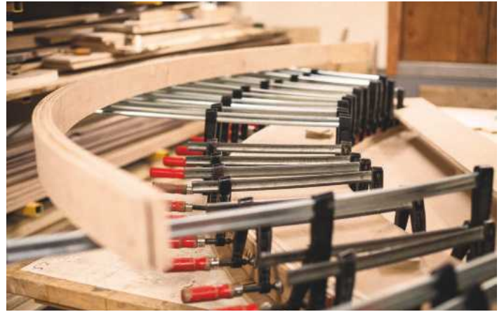
The suspended lighting hoop is laminated in sections. Note groove for lead string
