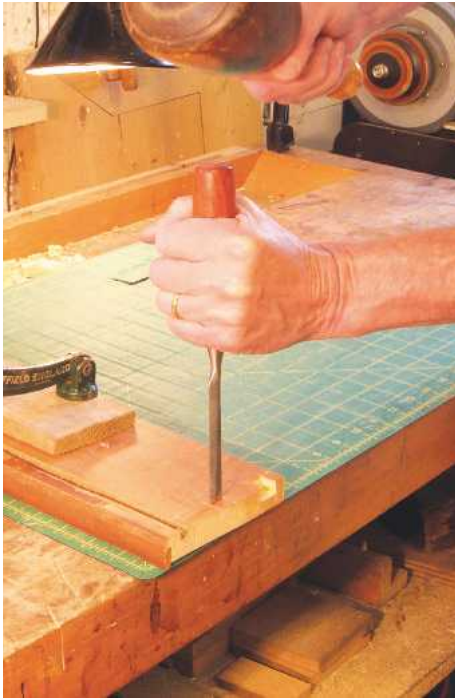
▲ Pic.10 Cleaning the lapped sockets going down first...
