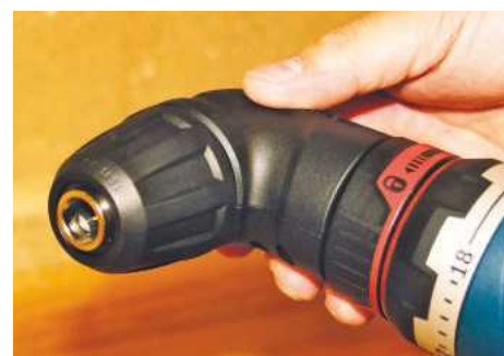
▲ For restricted areas the right-angle chuck is very handy
