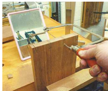
▲ Pic.7 Remove most of the waste for the dovetails with a coping saw and sharp chisel...
