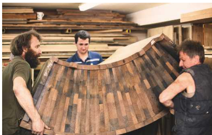
It's unlikely that Jack and his lads would make this lift look so easy if the sections were solid instead of hollow
