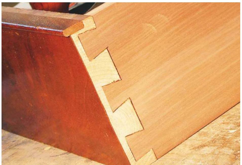
▲ Pic.13 The finished front-to-side drawer joint
