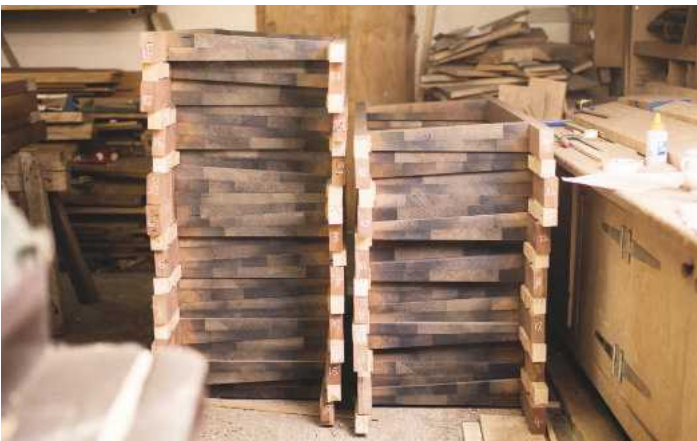
The machined frame segments stack up, fresh from the modified thicknesser
