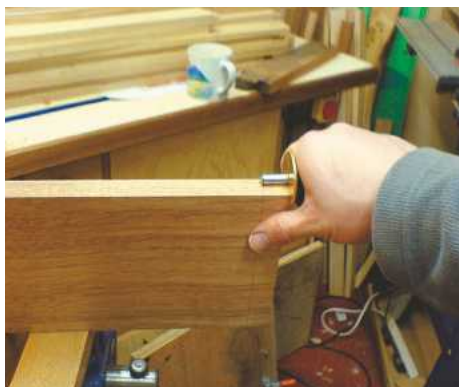
▲ Pic.5 Scribe around the boards to mark out the baselines for a set of dovetails
