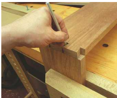
▲ Pic.8 ...after which you can use the tail board as a template when marking out the pins...
