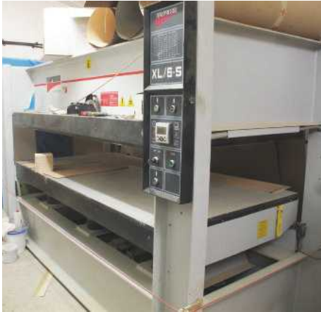
▲ Pic.1 Unless Les had access to a veneer press he wouldn't have taken this job on. To clamp everything would be too time consuming because of the quantities involved
