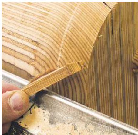
▲ Pic.17 Be aware that large pieces can splinter off as you are working through the curve. Make lighter cuts as you get nearer the finish shape to get the best finish off the tool
