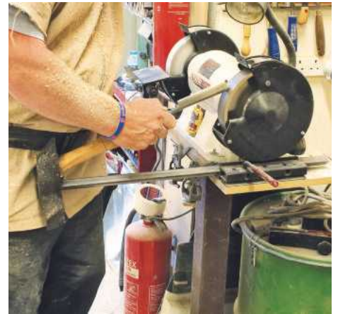
▲ Pic.12 Constant sharpening means that you will get the optimum cut. The Oneway jig makes touching up the edge of the roughing gouge simple
