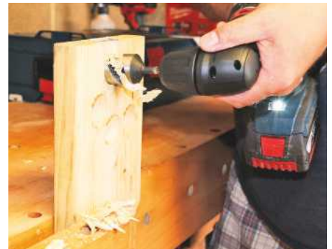
▲ There's also plenty of power on right-angle applications, easily drilling 32mm holes
