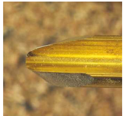
▲ Pic.18 You can just see the top wing on the gouge has been dulled off. As soon as you can see a cutting edge 'looking back at you' it's time for a sharpen
