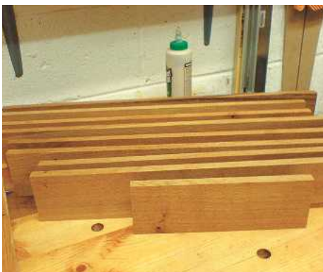
▲ Pic.17 You can then pre-finish the dividers, ready for final assembly
