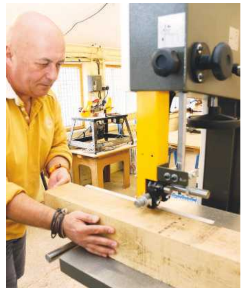
▲ Cutting this wet oak caused the saw to slow as it clogged in the cut
