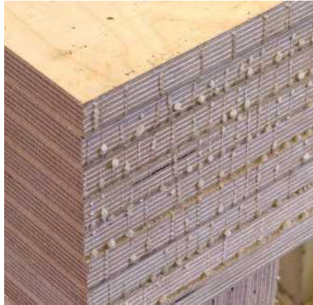
▲ Pic.2 The glue is UL39 formaldehyde, similar to the glue used in plywood construction, with a slow cure time that is perfect for laminate construction. 220 bar pressure certainly squeezes the excess out
