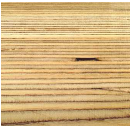
▲ Pic.25 You can now see the small voids that occur in the wood. There is little point in trying to turn these out as you will only find another one further down
