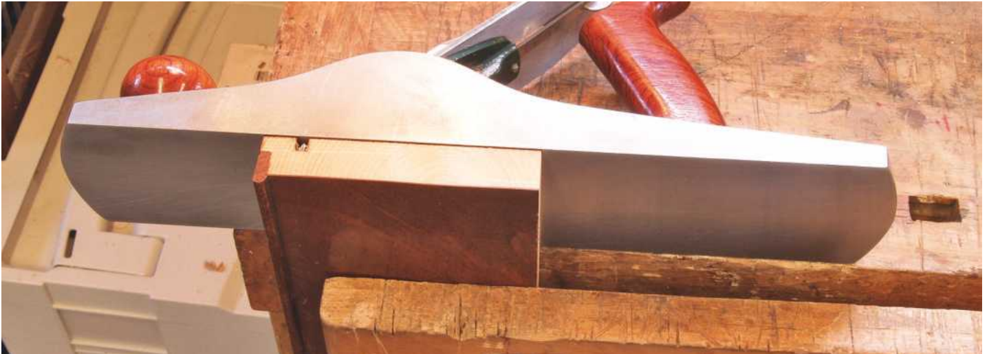
▲ Pic.2 Set up the pinboard in a vice to the same height as a plane on its side
