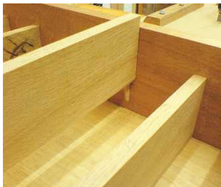
▲ Pic.15 Cut long slots using the biscuit jointer for the dividers and shelves to be slotted into
