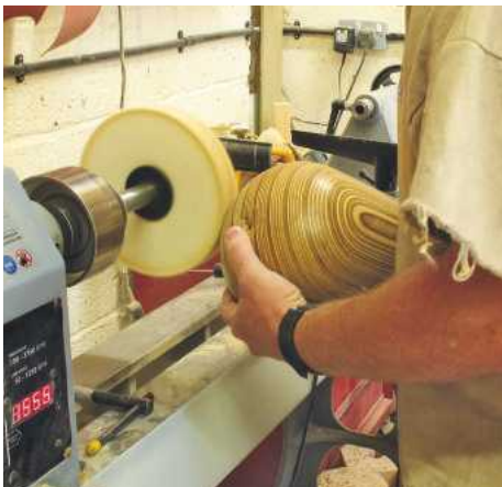
▲ Pic.31 You will have to hold on firmly if you decide to buff them to a nice sheen. He uses the brown compound on the hard wheel and then a light buff with the soft one
