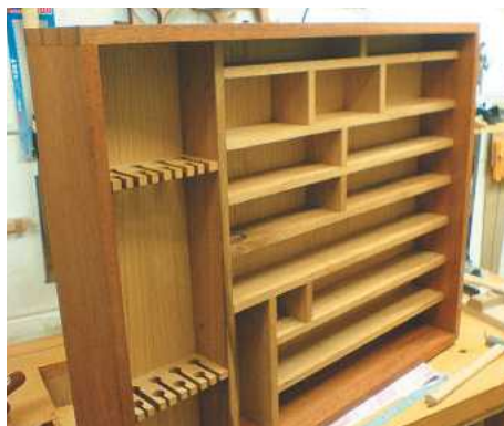
▲ Pic.18 The completed plane and chisel cabinet. Note the cut-outs for storing chisels
