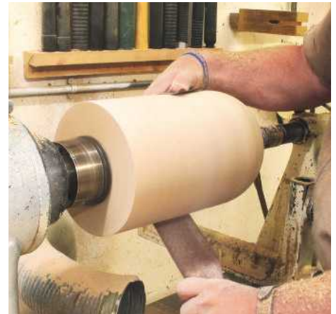
▲ Pic.21 You will find it very hard to get the desired finish off the tool so use the jokily named 60-grit gouge to finish off the shape. Plywood does sand remarkably well
