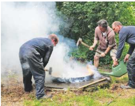
Wheelwrights thump a metal rim onto a wooden hub under fire, cooling with water from a can
