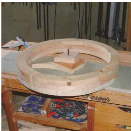
▲ Pic.8 With the frame attached to a board, build up offcuts until level and determine the centre
