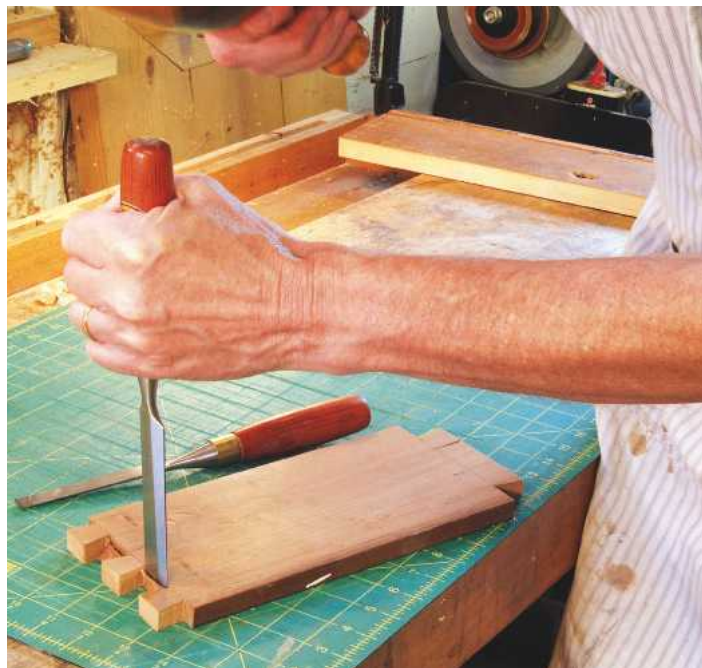
▲ Pic.9 Cleaning back to the shoulder line of the tails with a vertical cut
