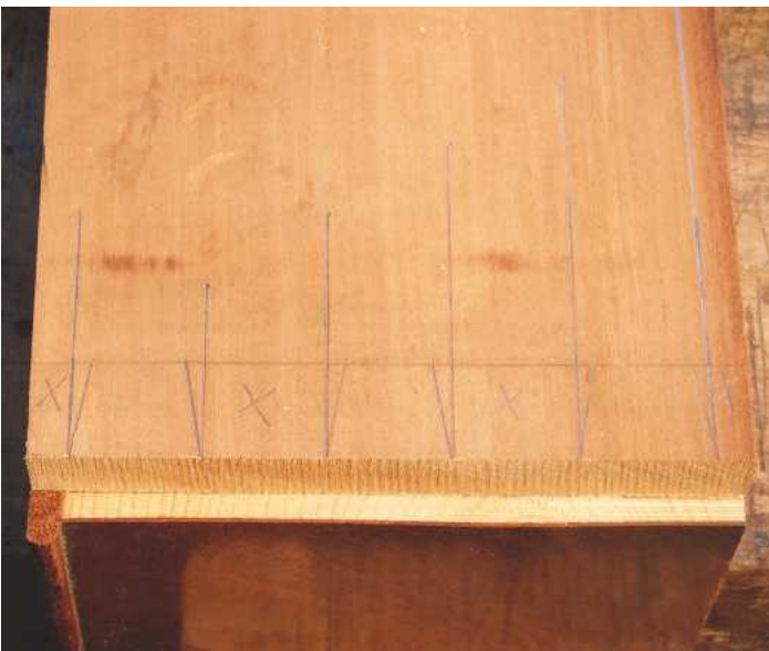
▲ Pic5 The tails marked out and the waste marked with an X
