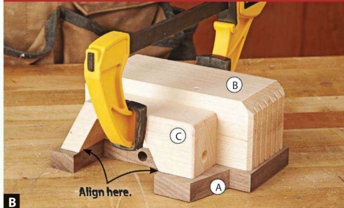
B Apply glue to the inside face of each front fender (C) and align the edges of the wheel well on the fender and the chassis (A).
