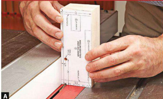
A Cut an outermost kerf first, then rotate the piece edge for edge to cut the opposite kerf. Reset the rip fence and repeat to cut the next pair of kerfs.
