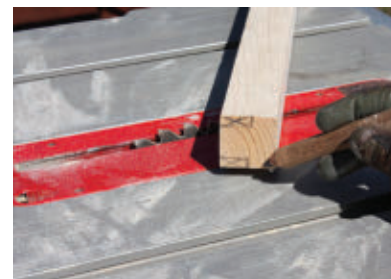
Measure and mark rabbets to seat the 1/4" plywood.
