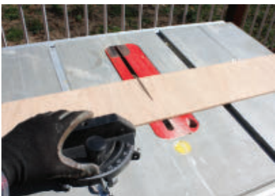
Trim the plywood to fit inside the groove.
