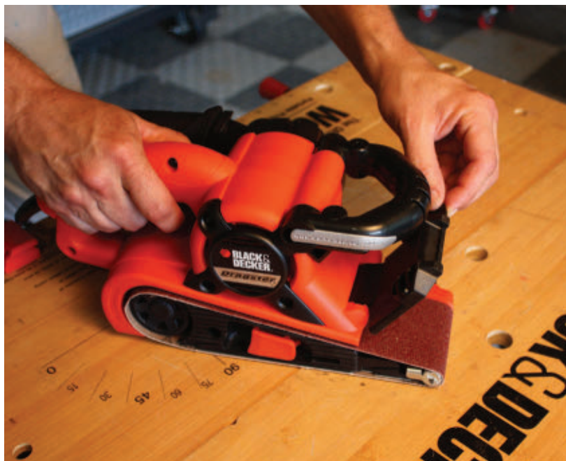
The Black & Decker Dragster belt sander has a low-profile nose and retractable guard that allow sanding in small spaces.
