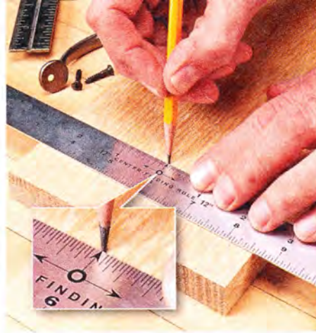
▲ This center-finding rule provides a reliable way to lay out hardware locations on the face of a workpiece.
