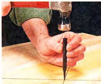
▲ To find the center, draw lines from the opposite corners and dimple the intersection.
