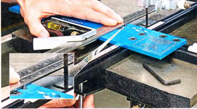
▲ Set up the jig so that the fixed rail is perpendicular to the miter slot, the crossbar is parallel to the miter slot, and the pivot pin is perfectly aligned with the front of the blade (above).
