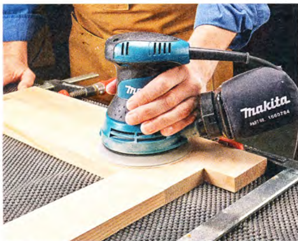
▲ To prevent rounded edges and ends when power sanding, clamp on "outriggers." These are scrap boards that match the thickness of the workpieces.
