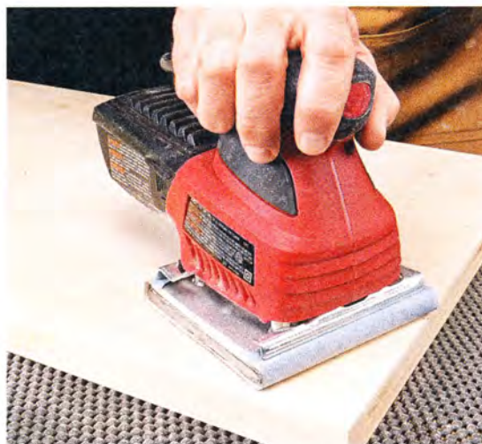
▲ The palm, or finish, sander, does have its place. I like to equip it with 180- or 220-grit paper for the final pass on flat panels or other wide workpieces.
