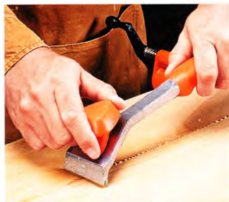
▲ A scraper is the ideal tool for cleaning up hardened glue. By using both hands, you can remove the toughest residue.
