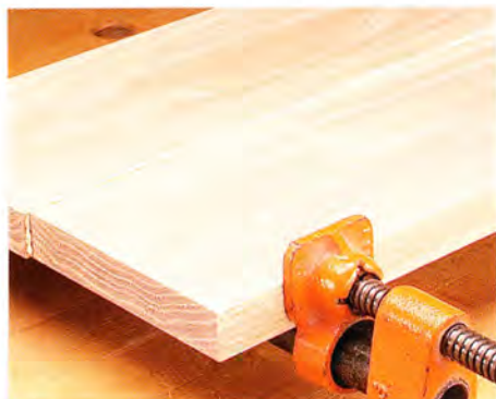
▲ Beads of glue on the joint line as you tighten the clamps are a good sign that you've applied the right amount of glue.
