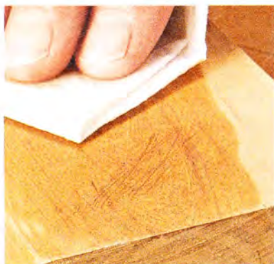
▲ A quick wipe of mineral spirits will reveal any surface imperfections without raising the grain.
