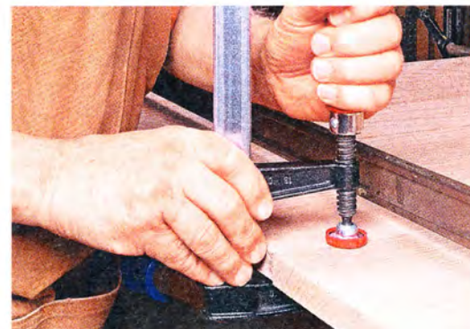
▲ Bar clamps are popular both for their reasonable price and high performance. Here, a small bar clamp levels two workpieces during an assembly.
