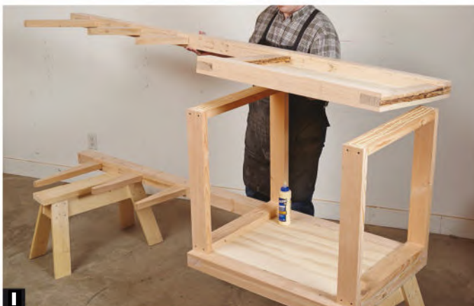
Attach the next upright assembly the same way. Check that the rear edges of the back uprights align along their full length. The second assembly will be a mirror image of the first.
