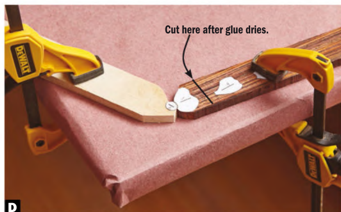
D Glue the first two parts. Cover your work surface with waxed paper or other nonstick material for assembly. Hold or clamp parts until the glue dries.
