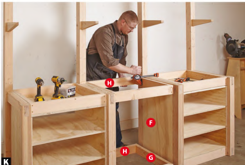
Tie the bays together. Screw, but don't glue, the two remaining frames (G/H) to the panels (F). This allows for disassembling the workcenter if need be.
