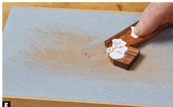
E Sand for a flat back. Flatten the back of the ornament as needed on a sanding block. A flat back makes scrollsawing easier as you assemble the ornament.
