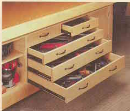
Bank of drawers. Keep your hand tools clean and organized in these generously-sized drawers. Plus, they open on full-extension slides so you can fill them from front to back.
