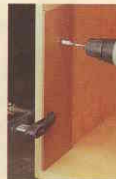
▲ A hardboard template allows you to accurately drill holes for the shelf pins.
