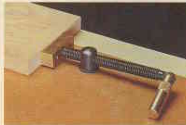
Wonder Pup. With its threaded shaft, the Pup serves as an end vise that can be placed in any dog hole.
