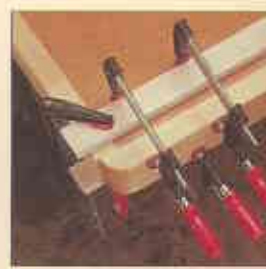
▲ A couple of cleats clamped to the top of the bench allow you to clamp the end aprons in place.
