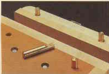
Round bench dogs. Put dogs in the bench top and vise, and you can clamp workpieces in a variety of ways.
