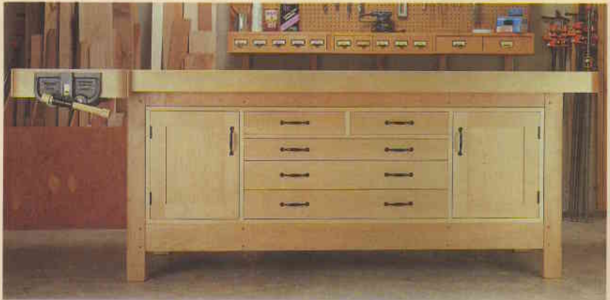
▲ Heavy-Duty Workbench. Modern materials meet traditional construction in this bedrock-solid bench. Three storage options include slide-in cabinets that can hold a shopful of tools. Step-by-step instructions begin on page 6.
