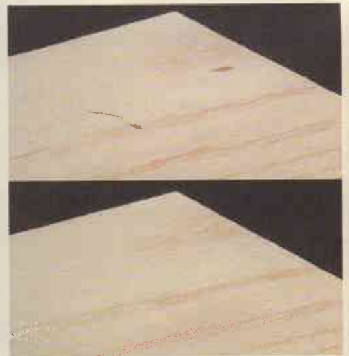
▲ With a little steam from a hot iron (see photo at left), the compressed fibers of a dent will swell back into place.
