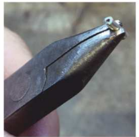
Cooperman ground these pliers with a bur to create a space to hold tiny pieces, such as this short section of sterling silver tube.
