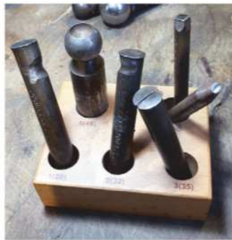
Andy Cooperman regularly customizes his tools, such as these dapping punches, to suit specific tasks.
