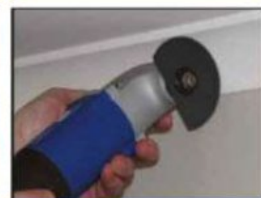
CUTTING PLASTER & CORNICE
