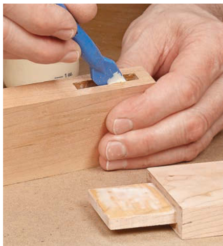
▲ For the strongest joint, brush glue onto the side walls of the mortise. No other glue is necessary for solid assembly.
