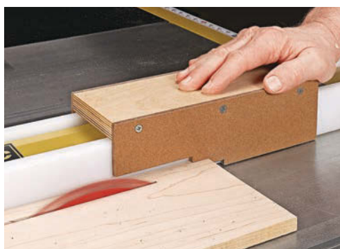
▲ This saddle is ideal for cutting narrow strips. Riding along the rip fence ensures that the piece you're cutting is moving in a straight line.
