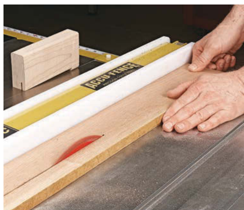
▲ Start cutting a long board by feeding the workpiece with your hands. The push block should be located within easy reach.
