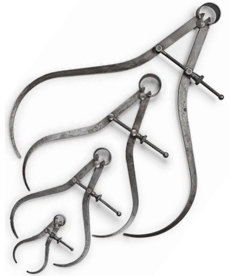
▲ Calipers are sized according to their maximum opening. They typically range from 3" to 12", as shown here.
