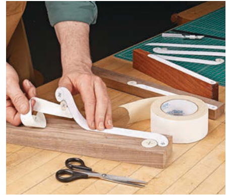
▲ Use double-sided tape to attach the plastic patterns to the blanks. The patterns can be easily removed and reattached as needed.
