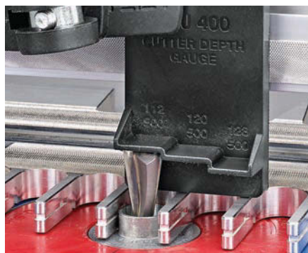
▲ A bit depth gauge makes it easy to set the height of the dovetail bit for cutting accurate half-blind dovetail joints.
