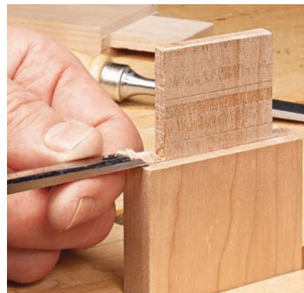
▲ Cure stepped shoulders by taking small bites with a chisel. Register the chisel on the low side of the shoulder.
