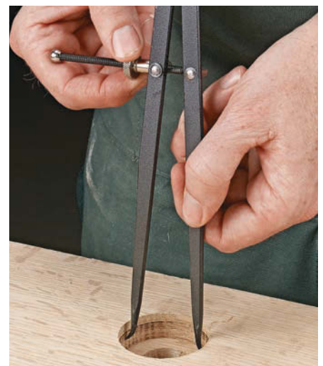
▲ A pair of inside calipers can be useful for gauging the diameter of a hole, recess, or other interior space.
