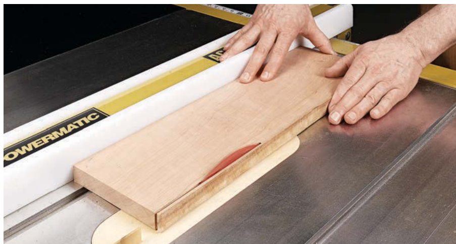
▲ When making wide cuts, your hand guides the workpiece. I like to hook my outer fingers over the fence rail to serve as a physical reference to make the cut safely.
