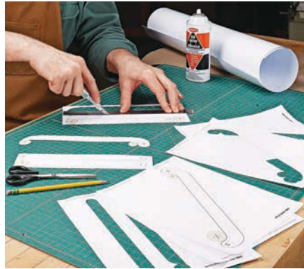
▲ High-impact polystyrene (HIPS) makes an ideal material for patterns. It's durable and cuts easily with a knife or scissors.
