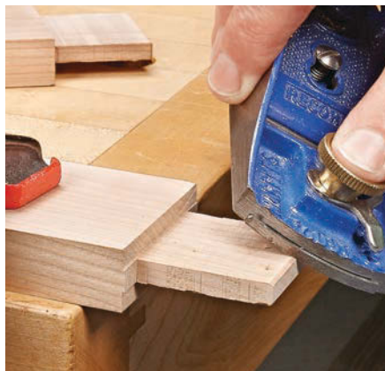
▲ A slight chamfer around the end of the tenon allows it to slide into the mortise easier, and it provides some glue relief.
