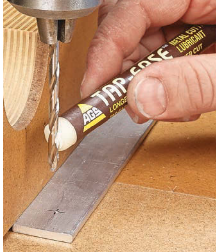
▲ Cutting sticks create a waxy barrier that helps keep drill bits cool and prevent chips from clogging up the flutes.
