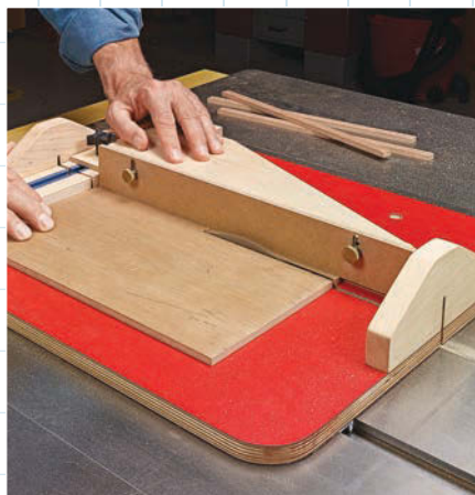
▲ Rip narrow, thin stock safely using the rip fence attachment with a built-in hold-down.
