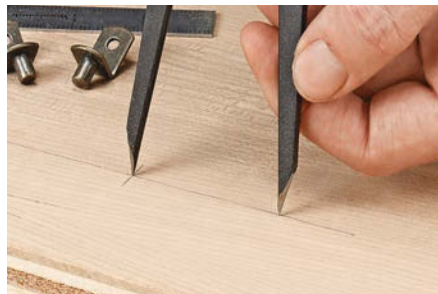
▲ A pair of dividers comes in handy for laying out equally spaced parts, joinery, or the locations for shelf pin holes.
