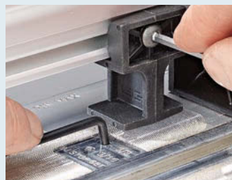
◀ Preset holes in the jig template allow you to accurately position the side stop for routing perfect-fitting box joints.
