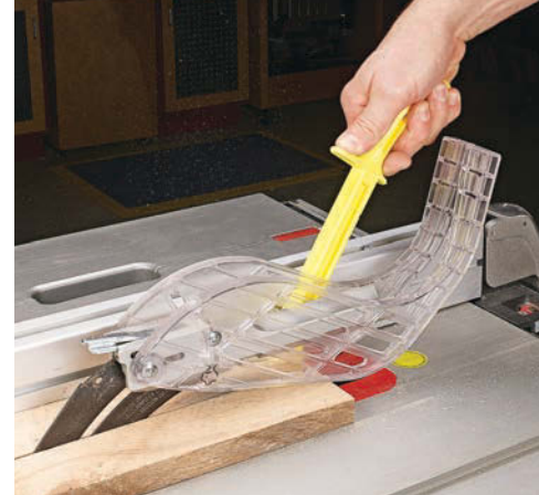
▲ A narrow push stick can fit between the blade cover and rip fence for all but the narrowest cuts.
