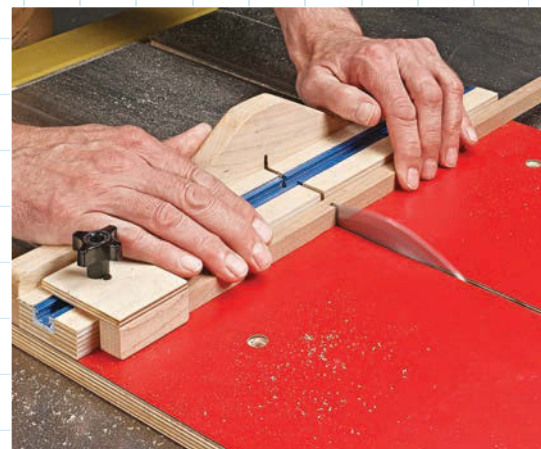
▲ A simple fence with a stop block makes square crosscuts on small parts a sure thing.
