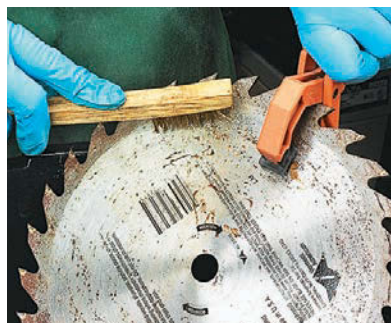
▲ All it takes is a few spritzes of blade cleaner to soften caked-on resin and pitch. The residue scrubs right off.
