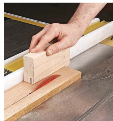
▲ Complete the cut with the push block. Lift your left hand from the saw table to keep it clear of the blade.
