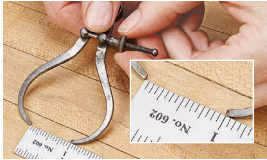
▲ To set a caliper to a specific size, place one leg against the end of a rule. Then open (or close) the other leg as needed. The knurled nut holds the legs in position.
