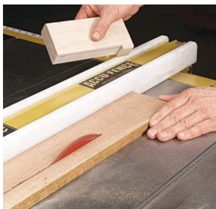
▲ Use your left hand to keep the workpiece moving slowly as you reach for the push block with your right hand.
