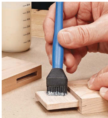
▲ Apply a thin, even coat of glue to the wide cheeks of the tenon. Too much glue here can lead to messy squeezeout.
