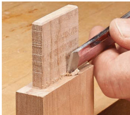
▲ A small ridge of waste where the tenon meets the shoulder can prevent a joint from seating. Trim it with a chisel.
