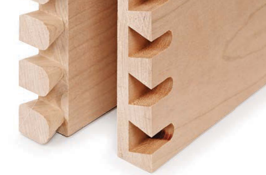
▲ With the Leigh jig, you can rout both the pins and tails of a half-blind dovetail joint in one operation.
