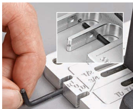
▲ For routing half-blind dovetails in thinner stock, you pass a stop rod through the template to limit the depth of the bit's cut.
