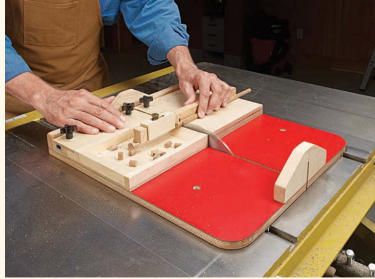
▲ Small Parts Sled . This scaled-down version of the classic table saw sled includes all the features you'd expect to find — plus a few more that are designed specifically for working with small parts. Plans begin on page 36.
