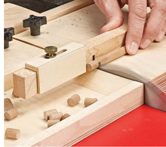
▲ The auxiliary fence platform and tray allow you to cut extra-small parts safely while collecting them in the tray.
