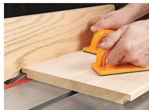
▲ Rubber-bottomed push pads give you a firm grip to hold the workpiece against the saw table.
