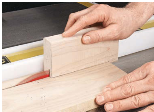
▲ A notched 2x4 push block makes for a simple, disposable guide. You can cut into the block while still maintaining control.
