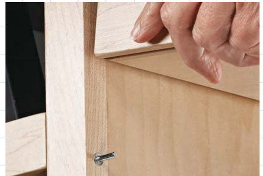
▲ Adjustable shelf pins make arranging the shelves a snap. The groove in the edging completely hides them from view.
