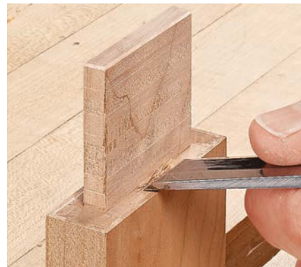
▲ Undercutting the shoulder all around the tenon is another method for eliminating gaps. Leave a narrow flat on the rim.
