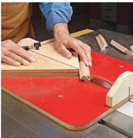
▲ Cutting miters on small frame parts is a snap with a pair of auxiliary miter fences.
