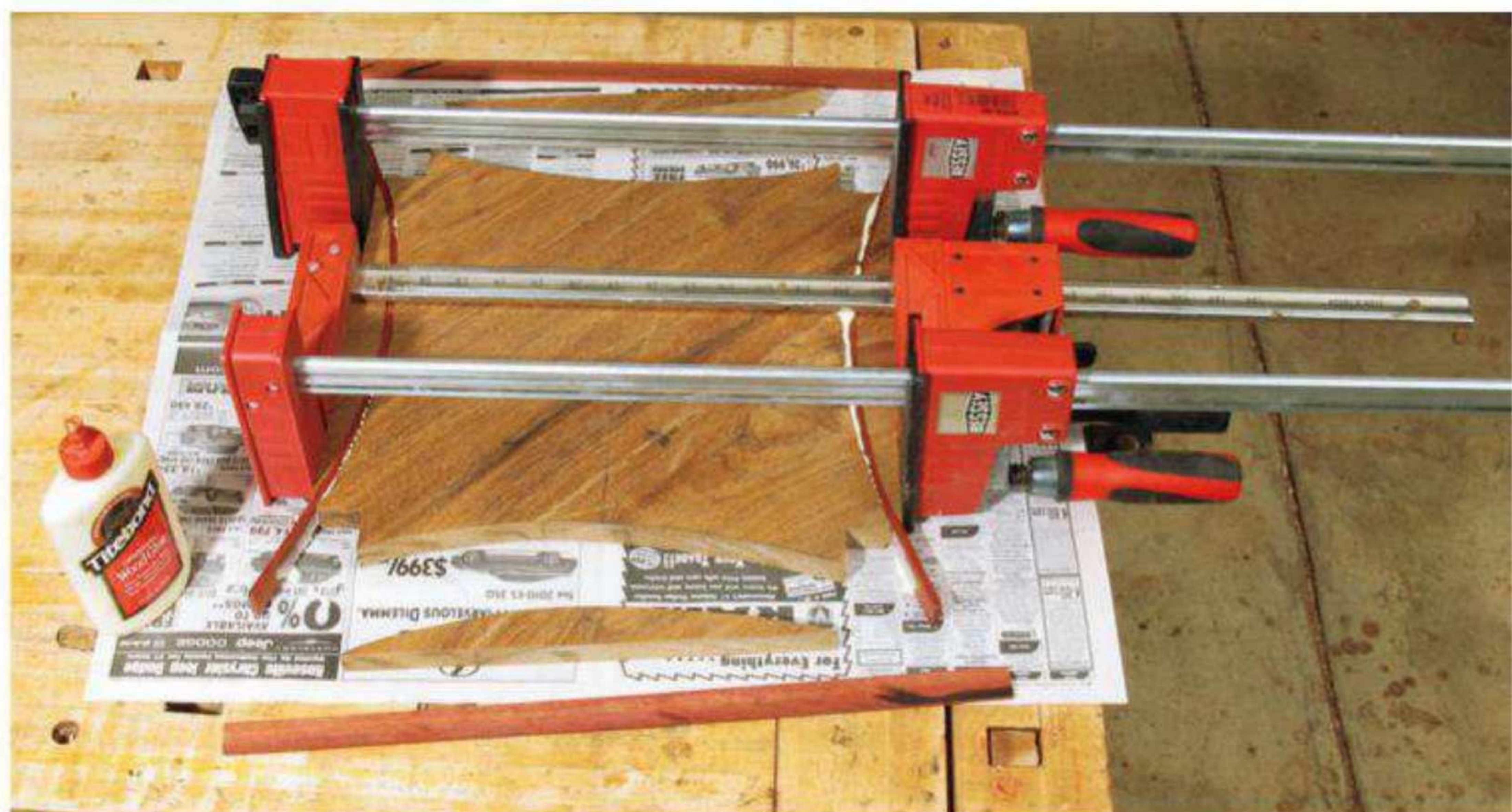
When gluing the strips to the concave shelf, the author reused his cutoffs as cauls to ensure that the joints received equal pressure along their full length. The strips are allowed to run long and then trimmed after the glue has dried. Given that the strips stand slightly proud of the top faces of the tabletop and shelf, choose a glue that can easily be removed once it cures.
