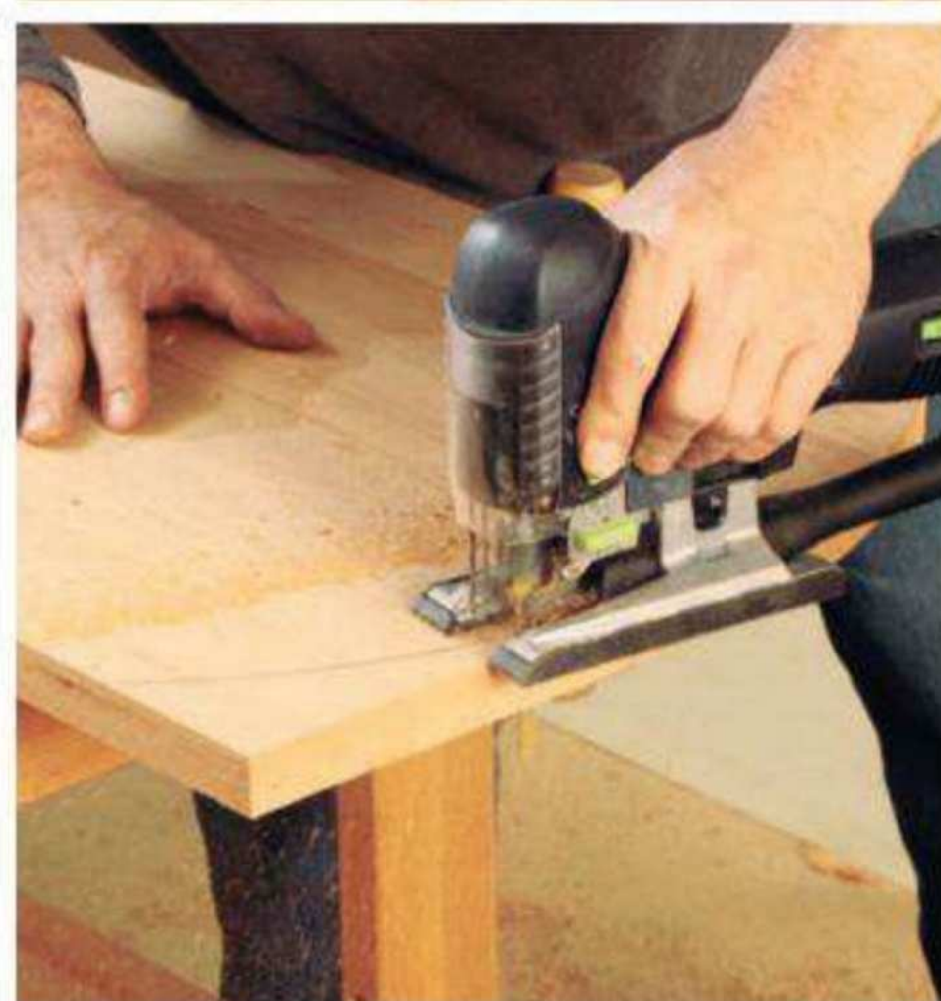
The glued-up top was the last piece to be completed. The curved radii were drawn with a trammel and cut out with a handheld jigsaw.
