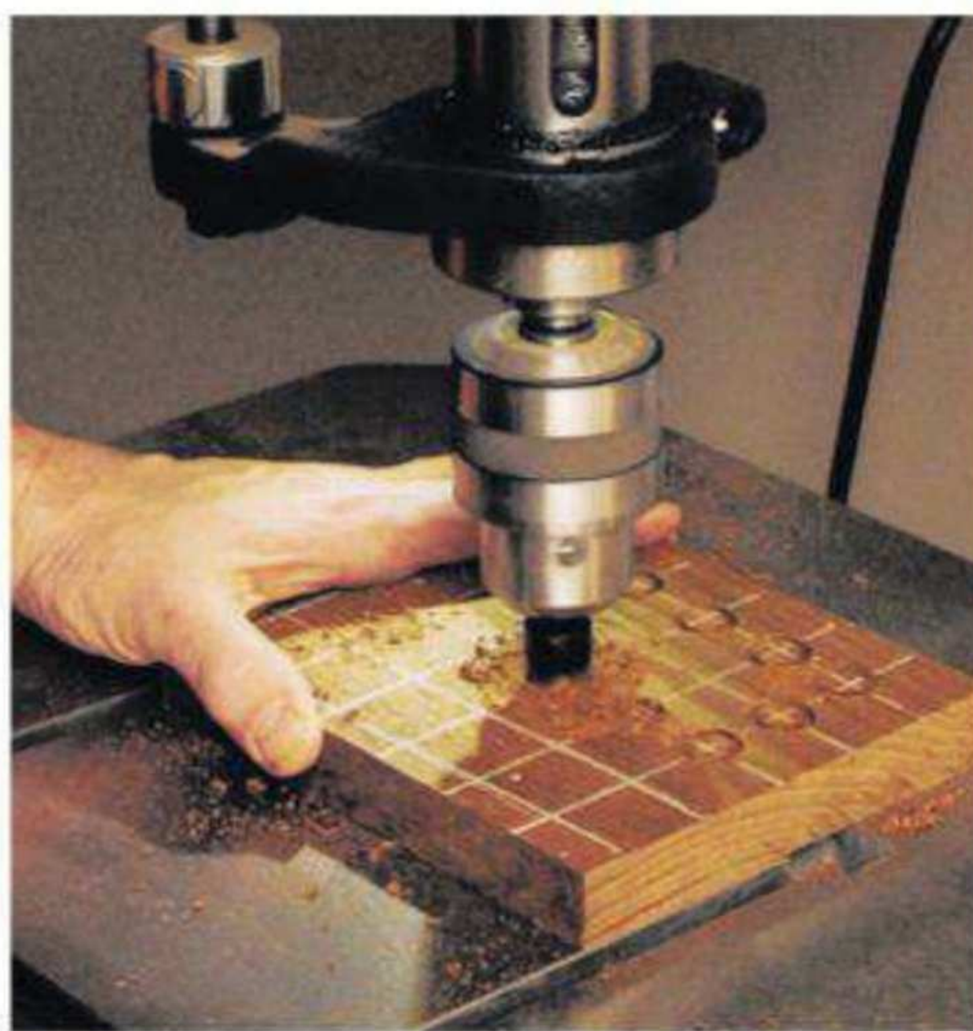
To match the color of the specially treated red oak, the author used a plug cutter to fabricate plugs from project scraps to cover the screws.
