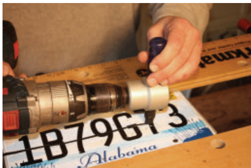
The Original Biter drill accessory is easy to maneuver with the steering handle.
