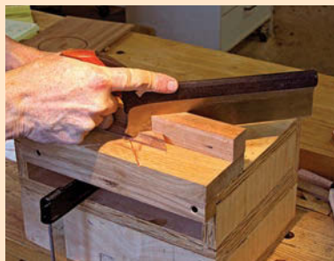
Simple solution. This shop-made miter cutting block (raised to a comfortable height) makes quick work of cutting the numerous miters for this project.
