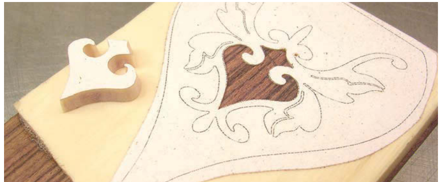
Tight fit. If you have the bevel on your saw table set correctly and make a good cut, the background piece will fit flawlessly.
