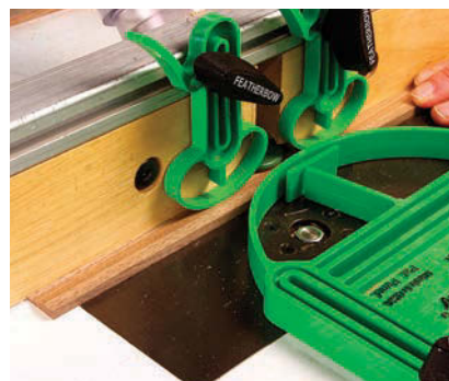
Second on face. The final cut leaves the narrow edge at a uniform thickness.
