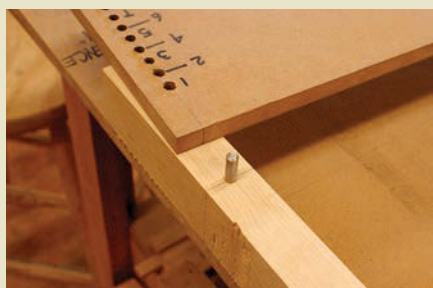
Bridge ahead. Place the bridge on the support blocks with the indexing pins in the No. 1 bridge holes.
