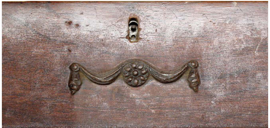
Crazed finish. Reviving a finish is a great solution in many situations where it has deteriorated. But be aware that the deterioration can be so bad that nothing short of stripping and refinishing can be done successfully. This example of a 100-year-old drawer front is such a case.
