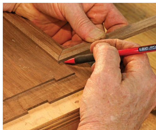
Slight return. The outside corners are used to mark the length of the moulding returns after the first miter is fit.
