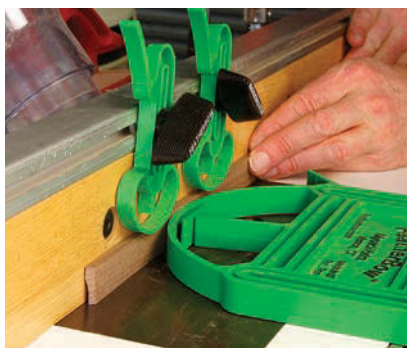
First on edge. The first cut of the cornice moulding is made with the wood on edge.
