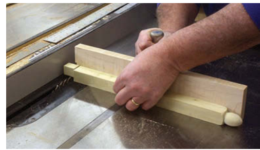
Accelerated & accurate. "Bump-cutting" the tenons at the table saw is a quick technique if you only have a few tenons to make.
