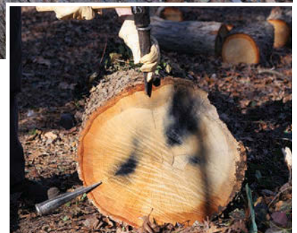
Get a handle on the material. I used the wedge in the 8 o'clock position as a handle to roll the log as I examined it. Once I had the log positioned, I set the first wedge to begin the split.
