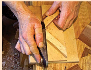
Shoot to fit. This fixture holds the workpiece at the correct angle and guides the block plane to perfect the ends of the mitered pieces.
