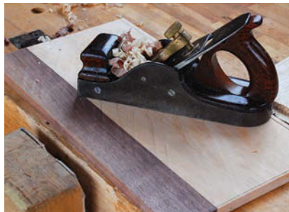
Waste not. Use primary wood only on the part of a piece that shows – in this case, the bottom panel of the top section. I glued up a walnut and pine panel to save my “good” wood for where it’s needed.
