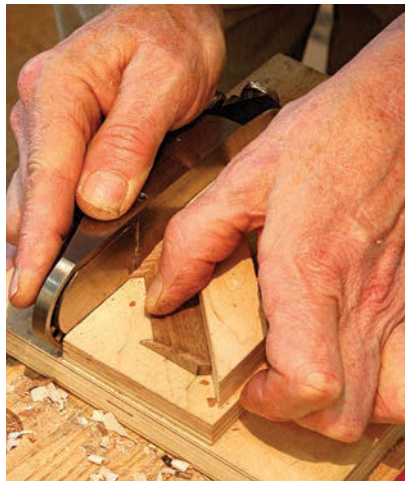
Handle it. The smallest pieces are glued to longer ones to make it possible to hold them for trimming the ends to the exact length.
