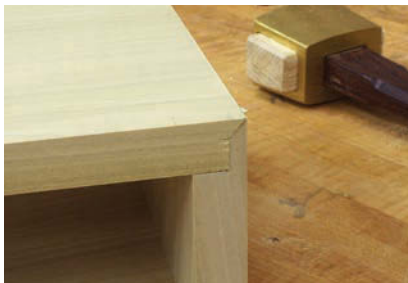
Twisted rabbet. The small bevel cut on the edge of the top rabbet eliminates end grain from the show surface.
