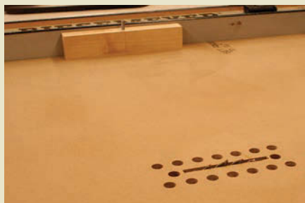
Get ready. To prepare for scooping, clamp the jig securely to the table saw then raise the saw blade to \frac{1}{8} " above the base of the jig.
