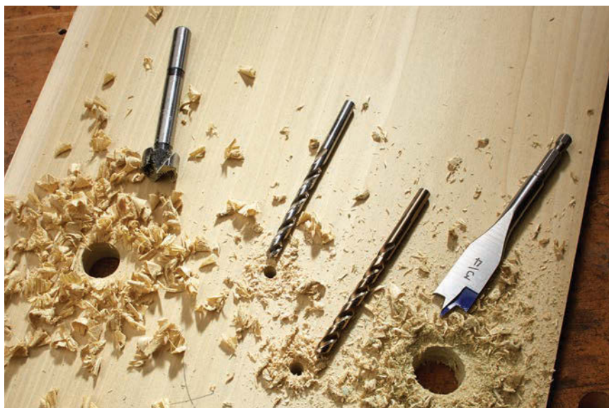
Pick your bit. All of these bits can drill holes in wood—so which should you choose? From left are pictured a Forstner bit, twist bit, brad-point bit and spade bit. See the chart on the next page for quick reference on using each.
