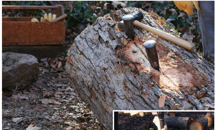
A gift from the storm. This 22"-diameter, 9'-long white oak log is from a tree felled in my yard by Hurricane Sandy. After splitting it, I'll be riving boards to use in projects for my home. Riven oak is perfectly radial and thus dimensionally stable and very strong.
