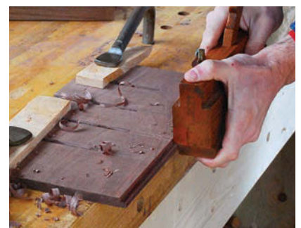
Rabbets. A moving fillister plane makes quick work of rabbets of many sizes, both with and across the grain, thanks to its retractable “nicker” and movable fence.
