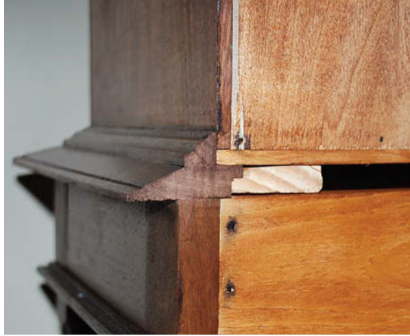
Case & stand connection. Two scraps with a rabbet on one edge are nailed to the bottom of the case on either side; they form a shiplap joint with a rabbet in the moulding on the stand. This setup holds the case and stand together.
