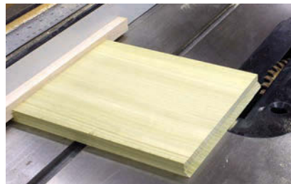
Simple fix. Because the mitered end can slip under the fence, a spacer set between the rabbet and fence allows one setup for both end cuts.
