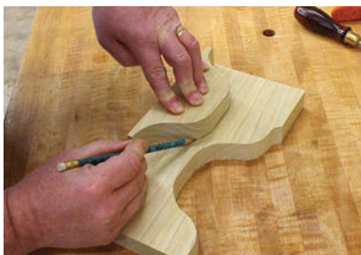
Base two. To make the second base side and get a matching part, it's best to work from your completed base than from the pattern.
