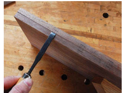
Size to fit. I use the same 3/8" chisel I'll use to cut the dados to define the dado shoulders. That way, I know I have the perfect-sized tool for the job.
