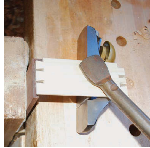
Half-blinds by eye. You can step off your dovetail layout with dividers, but doing it by eye adds a pleasing variation and guarantees a hand-cut look.
