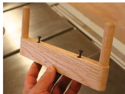
Get a handle. The guide block attaches to the bottom of the seat and controls the blank's travel along the bridge. Dowels serve as handles.
