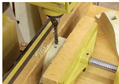
Squared hole. Cut a \frac{1}{2} " x \frac{1}{2} " mortise that is 1\frac{1}{4} " deep and centered on each post base at the crown of the piece.
