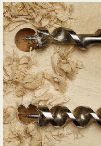
Two common patterns. The Irwin-pattern bit (top) has more widely spaced flutes than the Jennings-pattern bit. Note, too, the difference in the lead screws. The coarse lead screw on this Irwin is for softwood; the fine thread on this Jennings is for hardwood.
