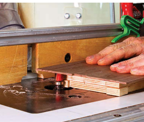
Follow me. The pattern is made to the exact size of the perimeter rabbet. The bearing on the bit follows the pattern to make the cut.
