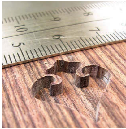
Mind the gap. Cut the background piece then press it down into the inlay piece.
