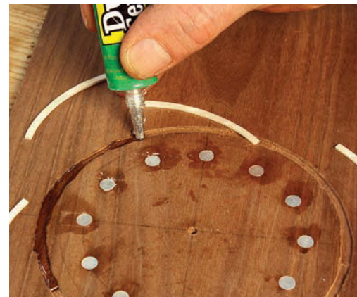
Drop in. The inlay materials were purchased as pre-cut parts from a luthier's supply store. These parts could also be fabricated from wood or other materials.
