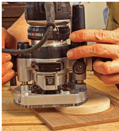
Take a turn. A plywood circle is used as a template for the router guide collar to follow when making the groove for the inlaid ring.
