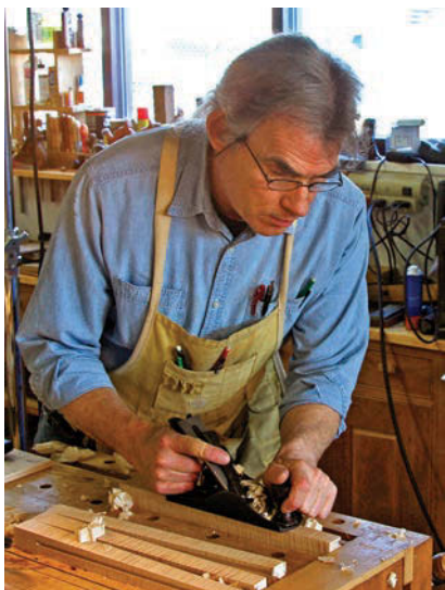
Smooth sailing. A handplane quickly removes the machine marks from the columns and it leaves a flat, smooth surface.
