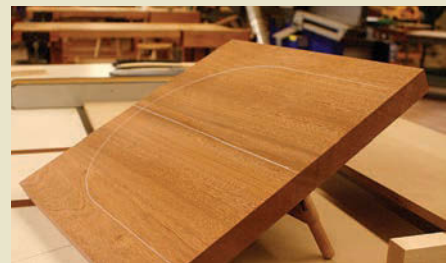
Hold on to your seat. The guide block is secured to the underside of the seat blank. It's held at the front edge and centered from side to side.
