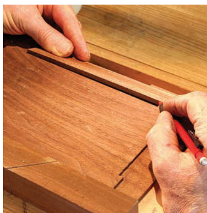
Start inside. The rabbet provides exact locations for the cornice moulding. The first piece fits within the notch.
