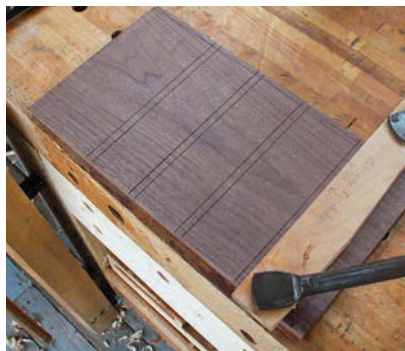
Saw guide. A straight piece of stock clamped at the dado shoulder helps to guide my saw for a straight cut.
