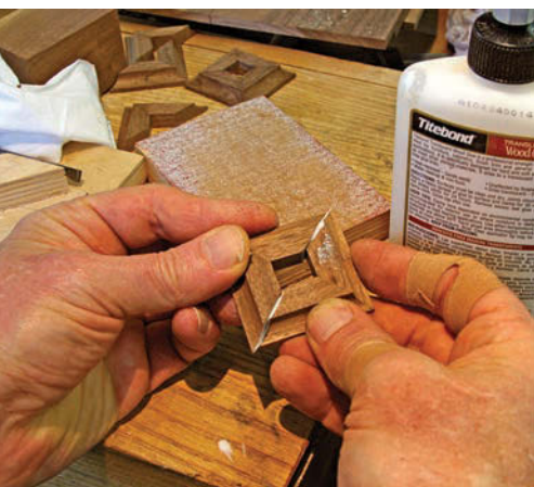
Two easier than four. Each half of a foot is put together, then two pairs are assembled to fit the tenons on the ends of the legs.
