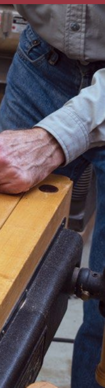
Stop-cut shoulders. When equipped with a stop, a crosscut sled ensures consistent tenon shoulders on the rails. Adjust the blade height just under your line so that you can sneak up on a perfectly fitting tenon.
