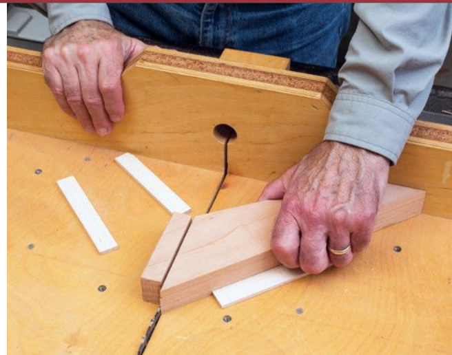
Sliding sled with custom stops. To cut the tenon shoulders on the angled feet, I pin-nailed stop strips to my crosscut sled. I then used my router table to cut the cheeks to fit the uprights.
