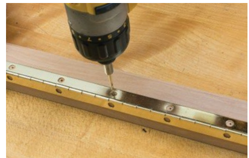
Hinge your frames together. To position the hinge, fold it over the stile, as shown. The "continuous" hinge requires two sections. Cut the hinge to fit the frame.
