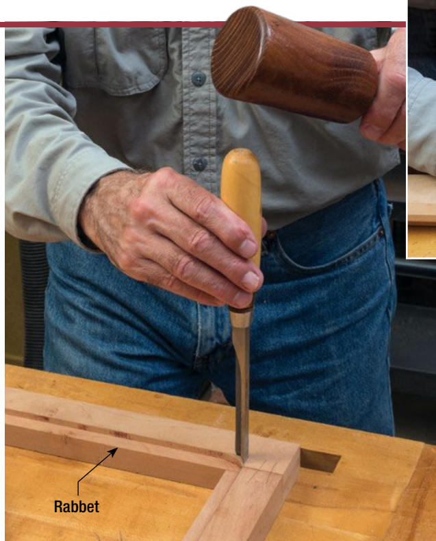
Chopped and sliced corners. Completing the routed rabbets and chamfers requires a little chisel work. To erase tool marks, I used a scrap of 100-grit sandpaper.
