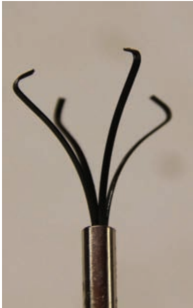
A prong retrieval tool has prongs on the end for grabbing objects in confined spaces.
