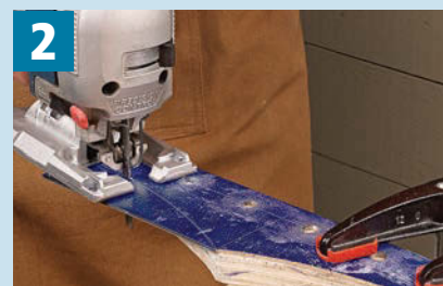
2 Arc Cut. With a metal-cutting blade in the jig saw, use a plywood backer to help cut through the mild steel.
