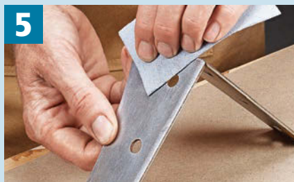
5 Sand. Sanding removes all the marking fluid and fingerprints from the surface of the metal in preparation for the patina.
