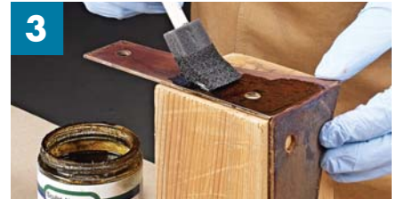
3 Topcoat. A foam brush is perfect for applying the oil topcoat. Give it two coats to protect the patina.
