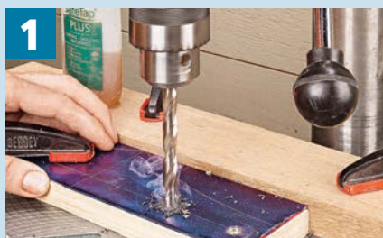
1 Drilling. After marking the shape and hole locations, drill the holes. I used a backer board to support the metal.
