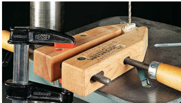
Since the clamp is a small piece and needs to be drilled precisely, secure it to the drill press table using a handscrew.
