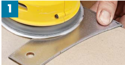
1 Rough-Up. I used 60-grit paper first, then 100-grit to sand the fresh metal and rough it up a bit for the patina.
