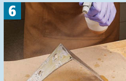
6 Patina. A spray-on patina is all it takes to for an aged look. For more on the two-step process, check out the Online Extra.
