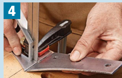
4 Bending. The scored line makes it easy to bend the steel. Use a square to guide you for a perfect fit on the corner.
