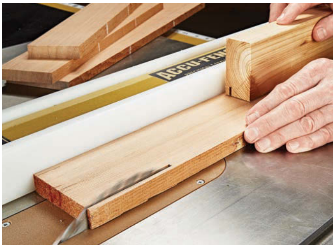
Rip. To get the second edge straight and parallel with the first, rip it a hair overwidth ( \frac{1}{32} " ) at the table saw. This way, you can make a single pass at the jointer to remove any saw or burn marks.
