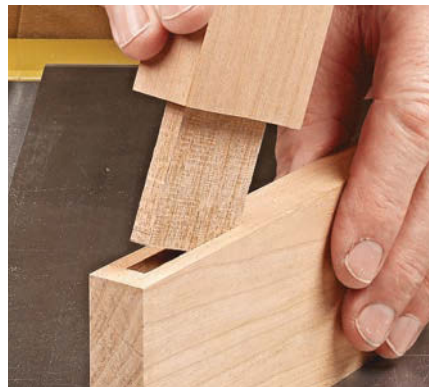
Fit. A properly sized tenon should fit into the mating mortise with moderate hand pressure or light mallet taps.
