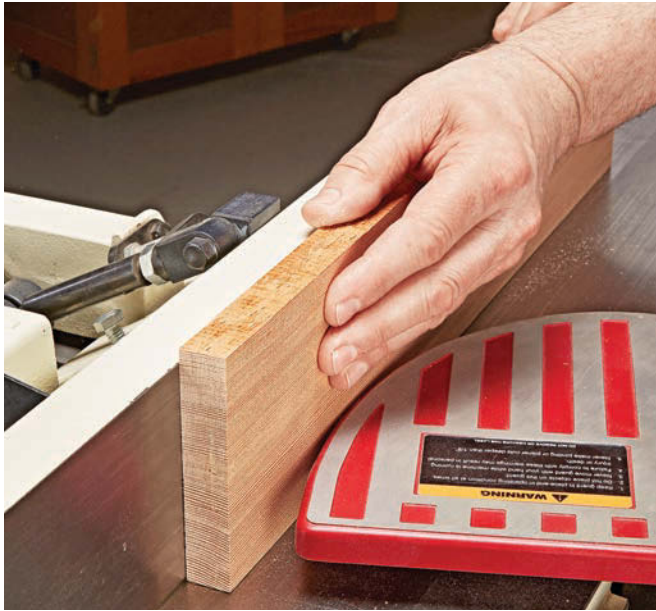
Joint Again. With the rough stock planed to final thickness, you can head back to the jointer to create one smooth, straight edge.
