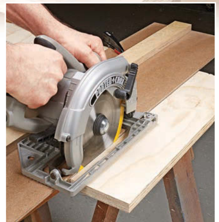
Dual-Use Jig. This simple, two-part jig can be customized for routing dados (main photo) or cutting sheet goods (inset).
