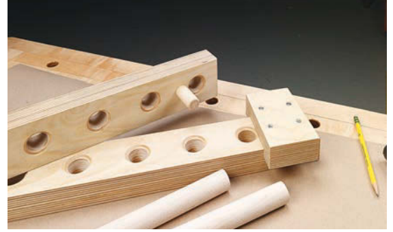
Dowels. A dowel recessed in one end of a base frame, and a cleat at the other end, hold them steady during use.
