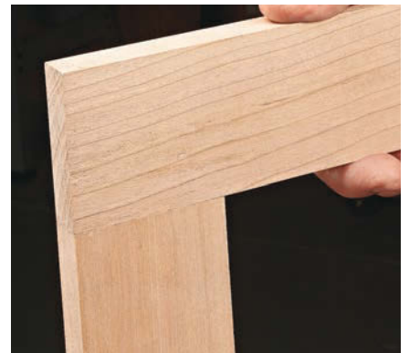
Check It. Another test for a tenon is to dry fit the joint and raise the mortised piece. The workpiece should stay in place.
