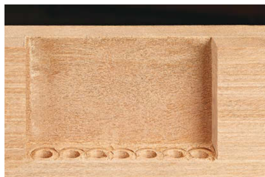
Paring. A wide chisel makes quick work of paring down the peaks left behind by the drill bit (top photo). Light, paring cuts result in a smooth-walled mortise (bottom photo).
