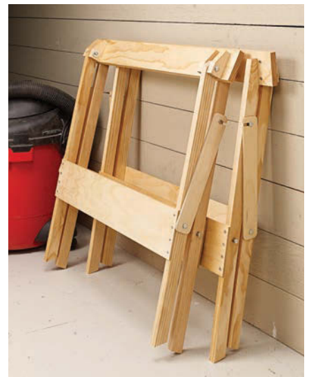
Compact. The sawhorses fold for storage. The braces hook onto a bolt on the leg to keep them locked in the closed position.
