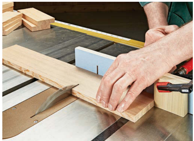
Crosscut. All that's left now is to cut the pieces to final length at the table saw. For workpieces that need to be identical length, use a stop block clamped to an auxiliary miter gauge fence.
