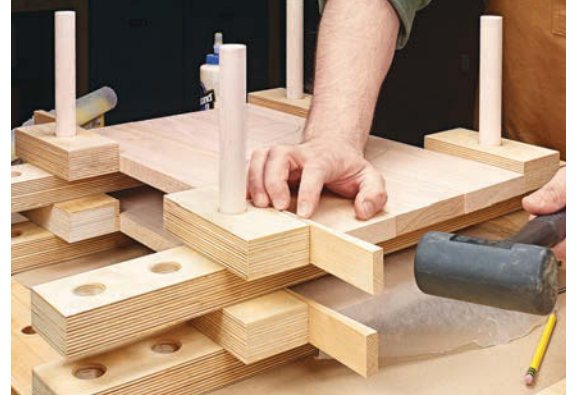
Multiples. Making multiple frames allows you to stack them vertically. The hardwood wedges secure the panels.
