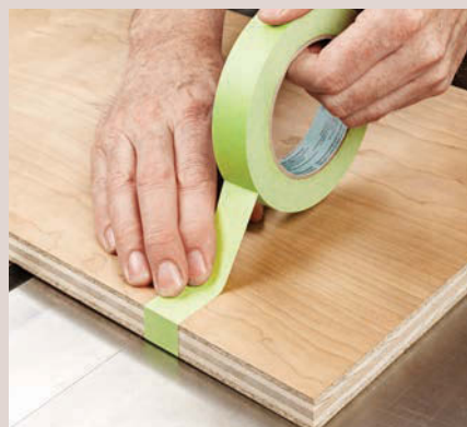
Extra Insurance. Masking tape placed on the cutline holds wood fibers in place to produce tearout-free cuts.
