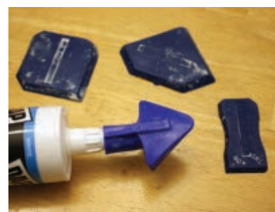
A number of caulk-shaping tools are available at most hardware stores.
